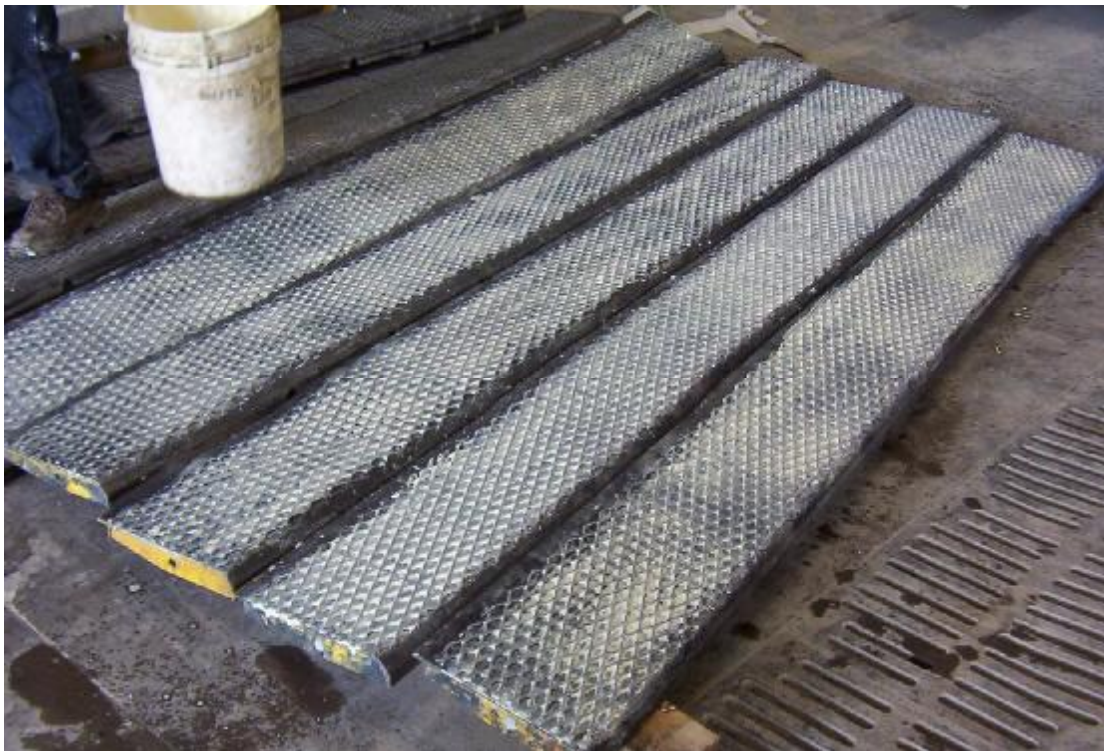
Figure 3.5 Photograph of formwork with indented inner surface
