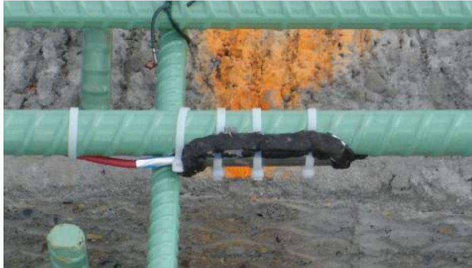
Figure 4.17 Photograph of VW spot-weldable strain gage with waterproofing and steel cover
