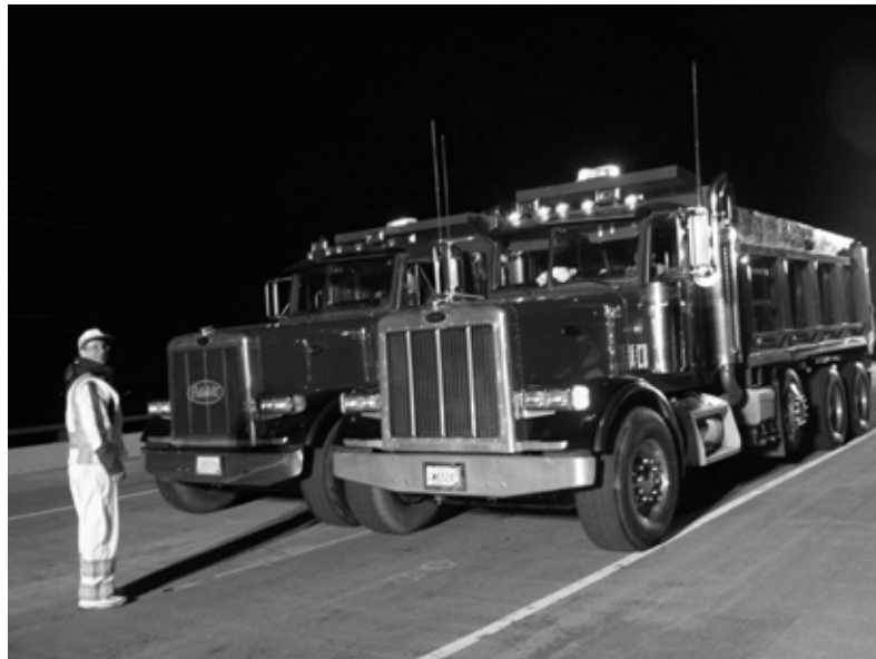
Figure 4.5: Photograph of the trucks during a paired position of the live load test
