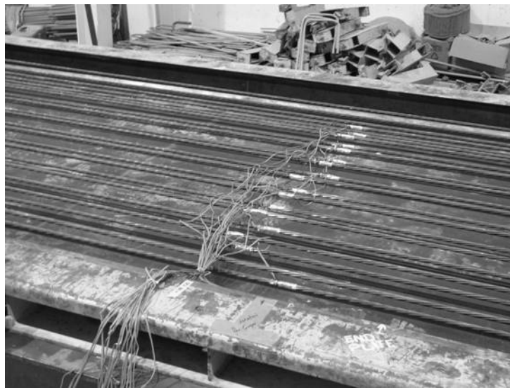
Figure 6.12: Resistive strand gages for measurement of initial prestress force
