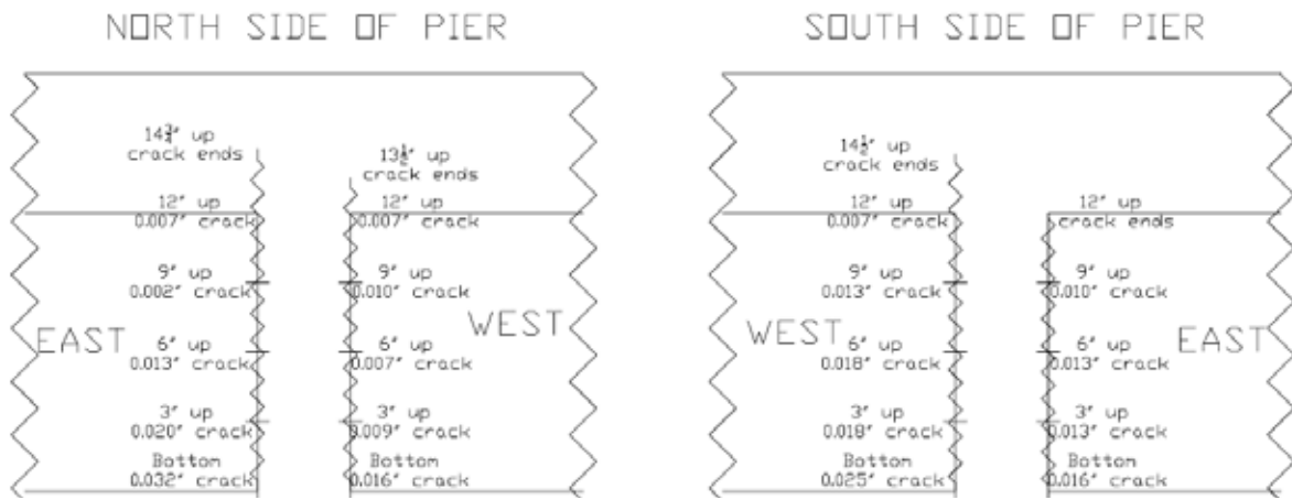
Figure 7.6: Cracking at pier observed during east load cell removal
