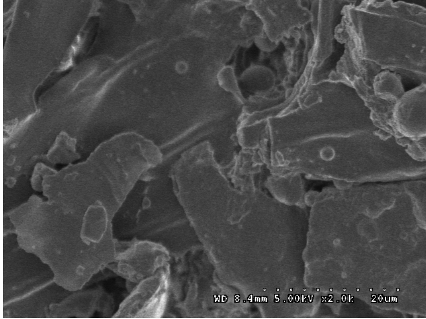
Fig. 13 2000× SEM image of HPH-C
