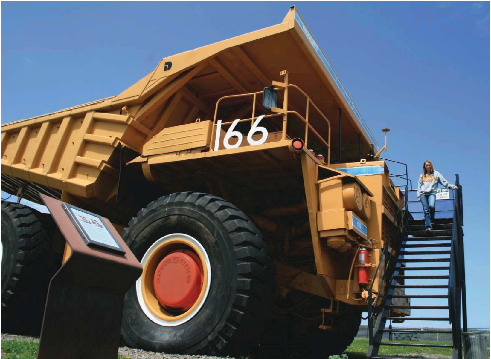
Fig. 4.18: Older Model 170-ton Haul Truck. Modern trucks are much larger 240+ ton models.
