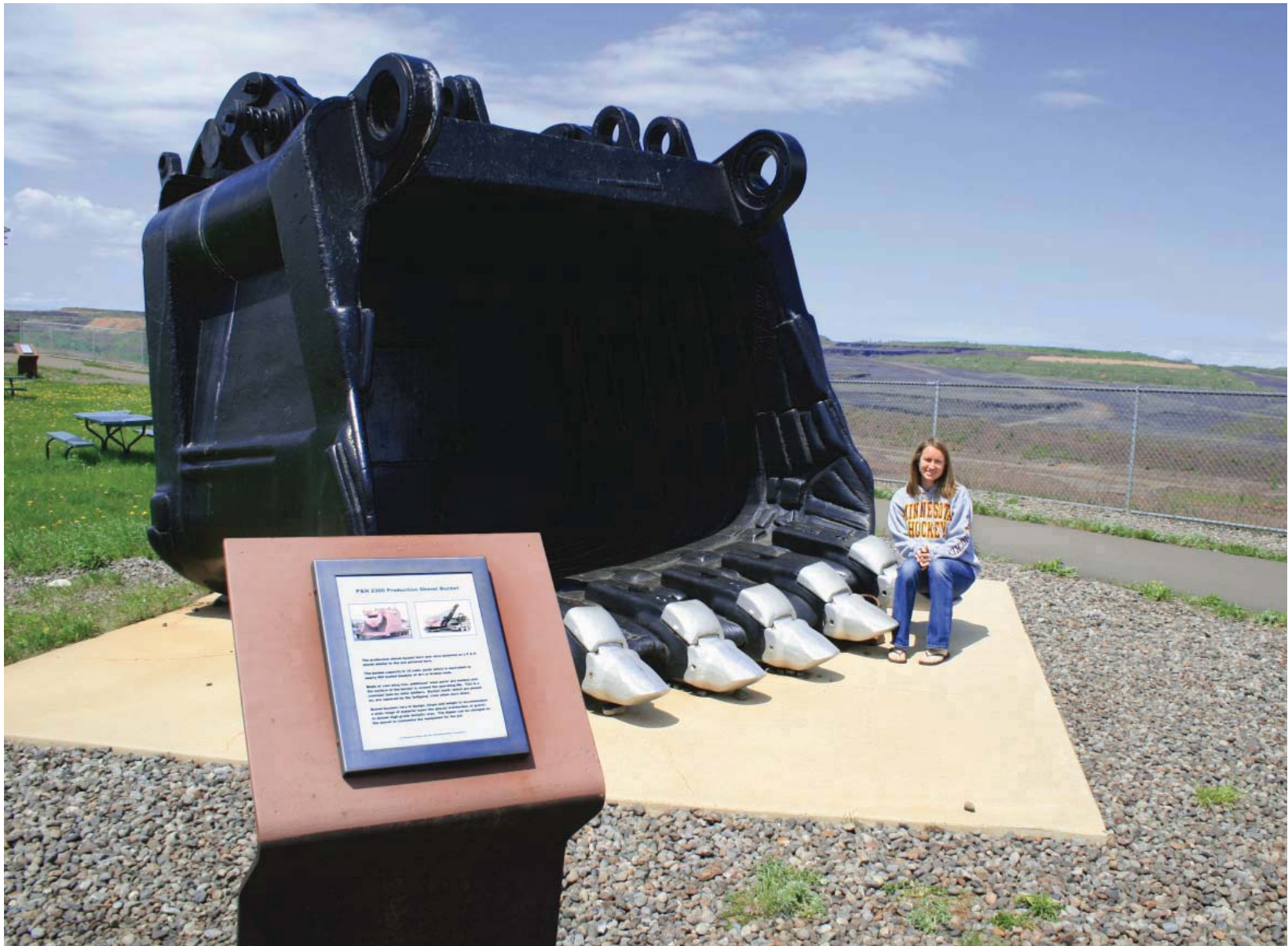
Fig. 4.19: Older Model 18-cu.yd. Bucket. Most modern shovels now use 34 cu.yd. buckets.
