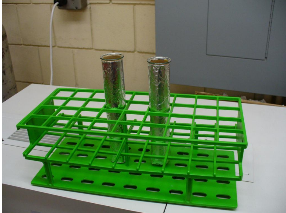
Figure 3-1. Test tubes used for indoor photolysis experiments with foil-paper cover.
