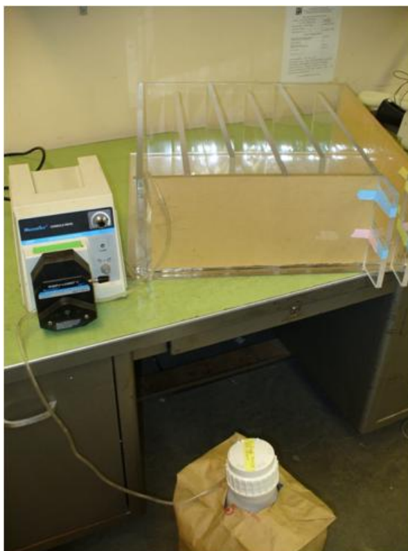
Figure 3-3. Solar reactor, peristaltic pump, and carboy.
