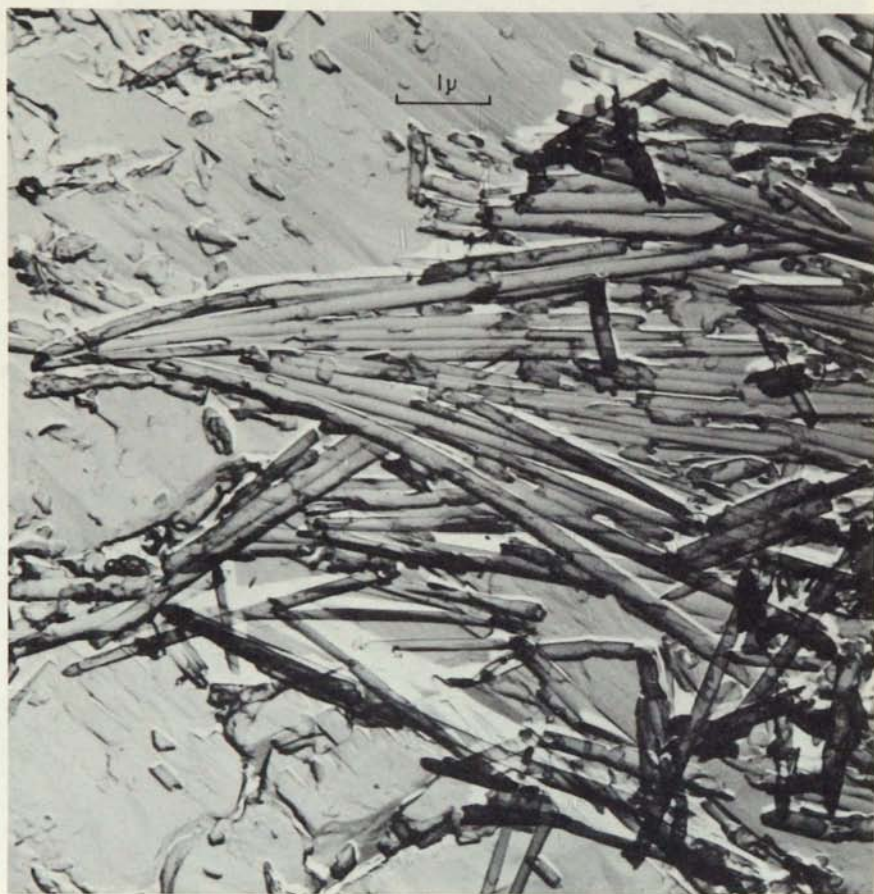
Figure 21. Carbon replica of halloysite on the inferred (010) cleavage surface of weathered microcline, Renville County, locality 74.
