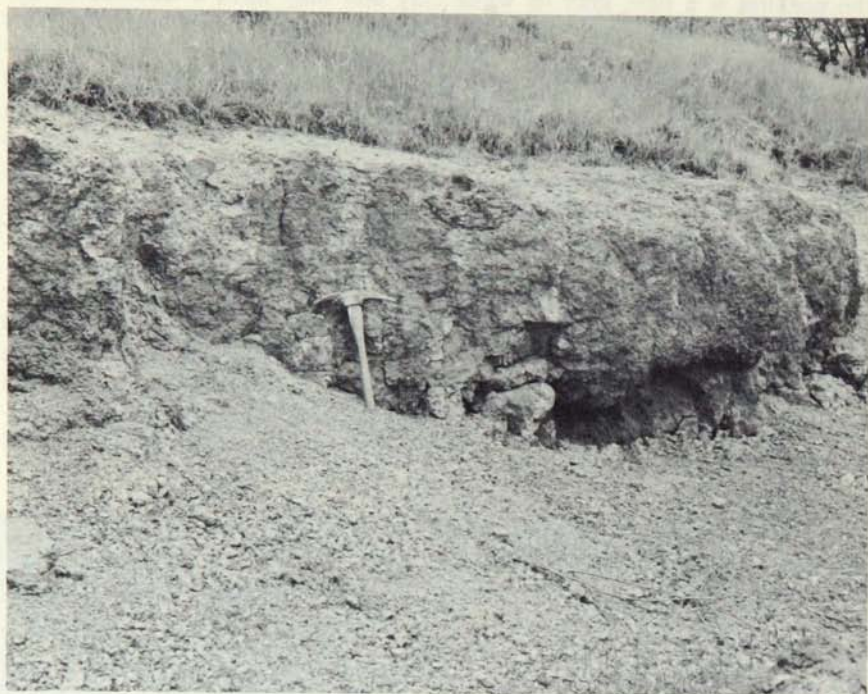
Figure 8. Upper Cretaceous hard, iron-rich, pisolitic kaolinite clay; forms ledges along valley walls of the Minnesota River and its tributaries, Renville County, locality 22. Pick length is 17 inches.
