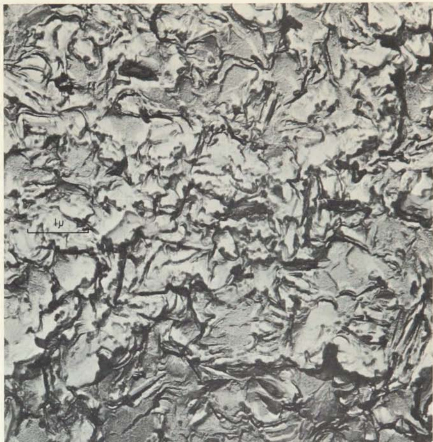
Figure 29. Carbon replica of poorly crystalline kaolinite matrix surrounding individual pisolites. Note lack of any well-defined pseudo-hexagonal outlines. Renville County, sample 42, locality 8.
