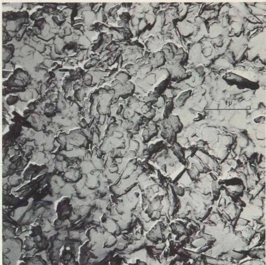
Figure 20. Carbon replica of a cleavage surface parallel to (001) of weathered microcline, Renville County, locality 74. Surface covered mostly with pseudo-hexagonal kaolinite plates.
