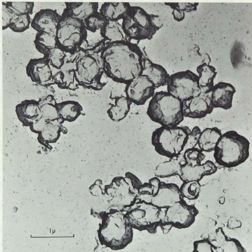
Figure 31. Carbon replica of spherical, platy halloysite from a thin white clay band beneath a unit 3 bentonite in clay pit, Redwood County, sample 69, locality 4.
