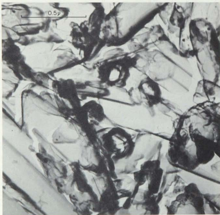
Figure 23. Carbon replica of halloysite developed on weathered microcline. Halloysite crystals have a prismatic form and a polygonal cross-section. Renville County, locality 74.
