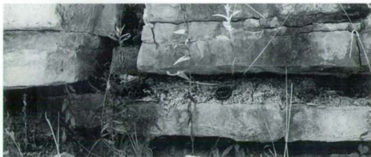
Figure 37. Bentonite bed, named the Deicke K-bentonite, near the top of the Platteville Formation at site 12. Bentonite bed is the clay seam marked by the camera lens cap.
