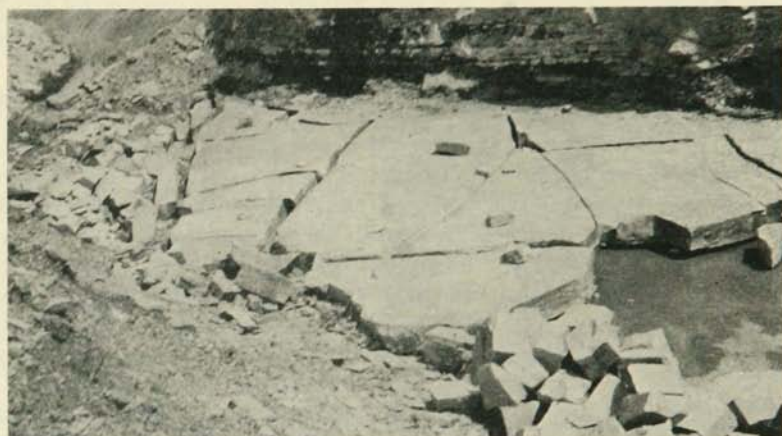
FIGURE 73.—The "marble" ledge at Lieb's Quarry, Faribault. The fracture pattern produces irregular slabs.
