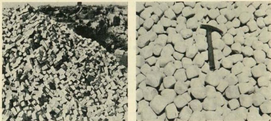
FIGURE 7. — Left: Quartzite blocks for lining grinding mills. Right: Quartzite pebbles for grinding mills.
