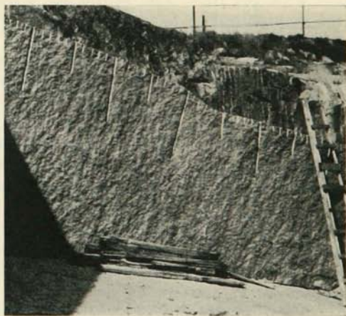
FIGURE 18.— Vertical fractures produced by plugs and feathers at the Royal Granite Company quarry, St. Cloud. Left: Short plugs and feathers of uniform length. Right: Plugs and feathers of three different lengths, 6, 18, and 36 inches, respectively.
