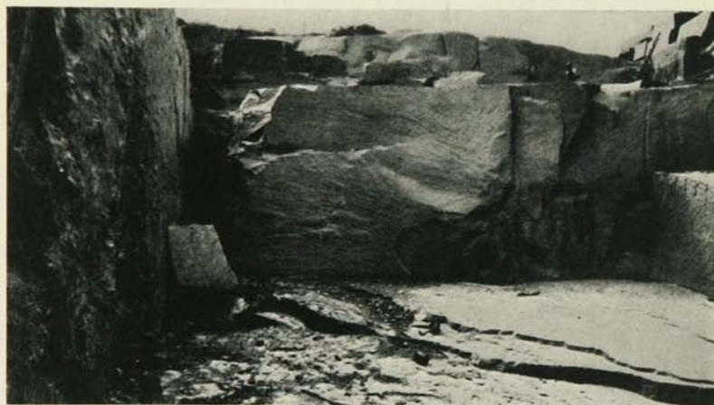
FIGURE 45. — The west quarry face of the quarry of the Royal Granite Company near St. Cloud. Two joint systems cut the rock at approximately right angles.
