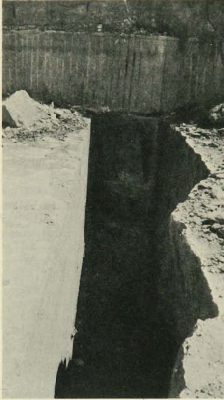
FIGURE 65.—An irregular "natural" fracture on the right and a straight channeled face on the left. Quarry of the Fowler and Pay Stone Company at Mankato.
