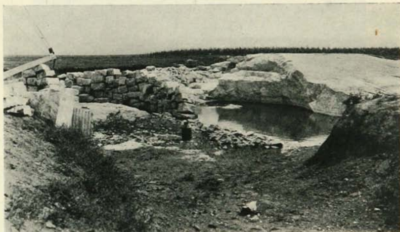
FIGURE 52. — Quarry of the Clark Granite Company near Seaforth. The rock is a light gray biotite granite gneiss.
