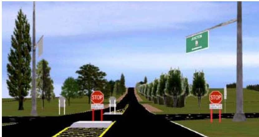
Figure B-6. Traffic islands, two STOP signs with reflective posts as countermeasures on the minor-road approach to the simulated intersection.
