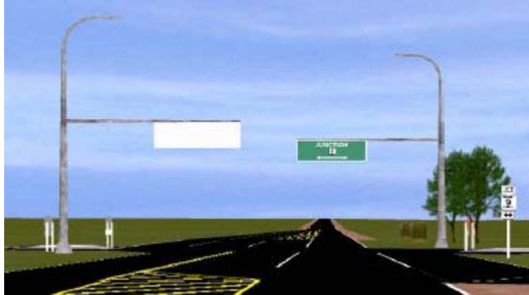
Figure B-7. Guide signs across the major road as countermeasure on the major road approach to the simulated intersection
