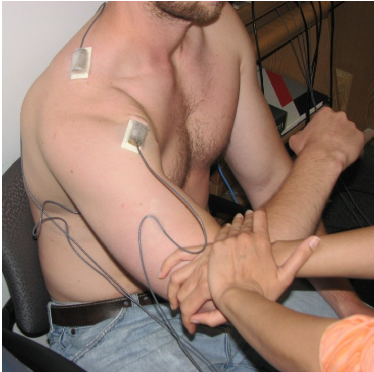
Figure 3.3 a: Position for recording maximum voluntary contraction (MVC) for upper trapezius and anterior deltoid.
