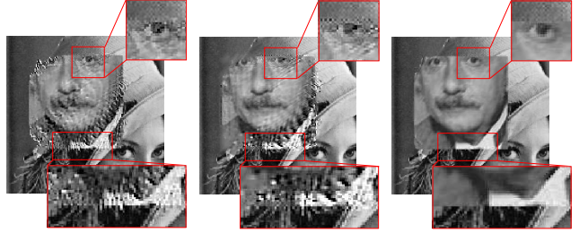
Figure 7. A comparison of our joint method with a non-joint method and with a method not taking into account the consistent motion blur model is shown. A restored frame with two zoom up areas is depicted for a straightforward scale variant motion deblurring, where the contour is extracted a priori based on pure motion competition (left), for the non-consistent motion blur model on the same a priori computed contour (middle), and for the fully joint method with the consistent model (right).
