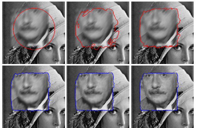
Figure 3. For the example from Fig. 2, intermediate results from our algorithm are depicted. In the top row from left to right the object contour is shown for three iterations from the initialization phase based on motion competition without deblurring. On the bottom three follow-up iterations of the joint method including the restoration of the frame are depicted.
