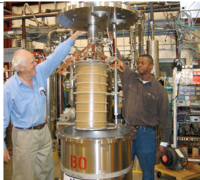
TPC being lowered into its cryostat
