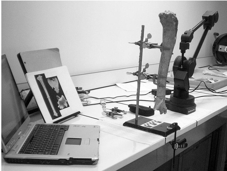
Figure 6-1 Set-up of the Microscribe MLX. Bunsen burner test tube clamps were used to keep specimens immobile. The Bunsen burner test tube holder was clamped to the table with a C-clamp. 3D coordinates were transferred from the Microscribe to the computer with a foot pedal.
