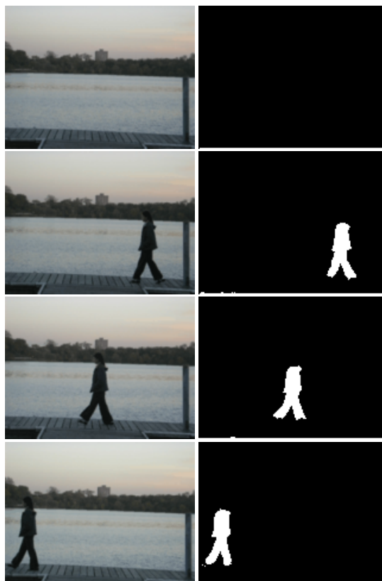
Figure 4. The dynamic background contains motion of water with wind. Considerable camera shake can be observed (please see uploaded videos). Original frames (# 0, 66, 82, 107) are shown on the left, while corresponding outliers detected are shown on the right.
