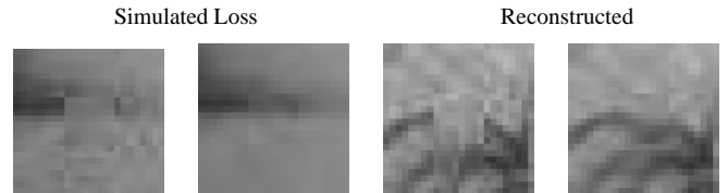
Fig. 5. Reconstruction of Lena with PSNR = 32.422 db. The bottom row shows details (hair and shoulder) of this image and the comparison of our technique (2nd and 4th) with the one by Hemami et al. (1st and 3rd).
