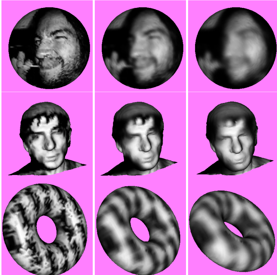
FIG. 1. Intrinsic isotropic diffusion (from left to right, original followed by two diffusion steps). Top: gray-scale image on a sphere. Middle: gray-scale image on the surface of a head. Bottom: synthetic scalar data on a torus.
