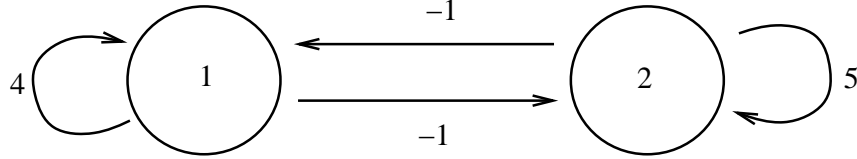
Figure 2: A two-dimensional recurrent network with six fixed points.
