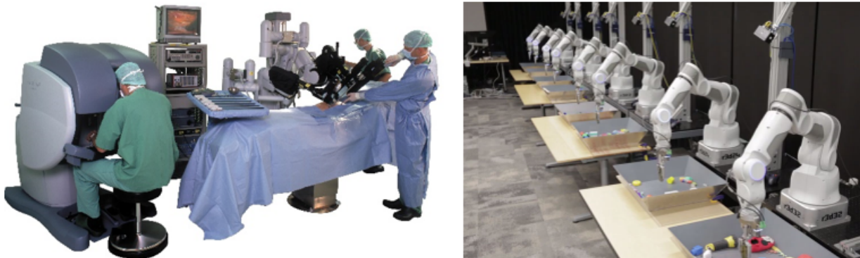
Figure 4.8: The Davinci surgical robot and a reinforcement-learning based robot locomotion from Google [20].
