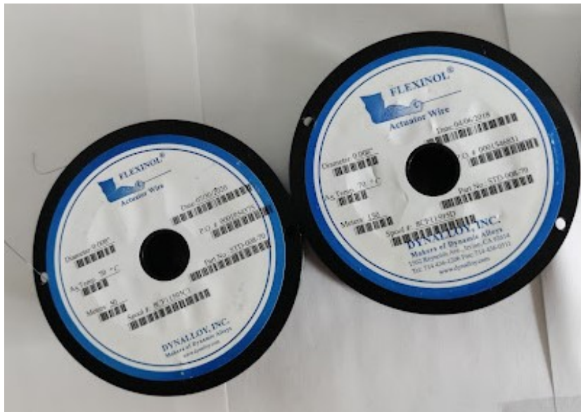
Figure 3.1: Dynalloy Flexinol wire spools for 0.006" and 0.008" wire diameters and transition temperature = 70^{\circ}\text{C}
