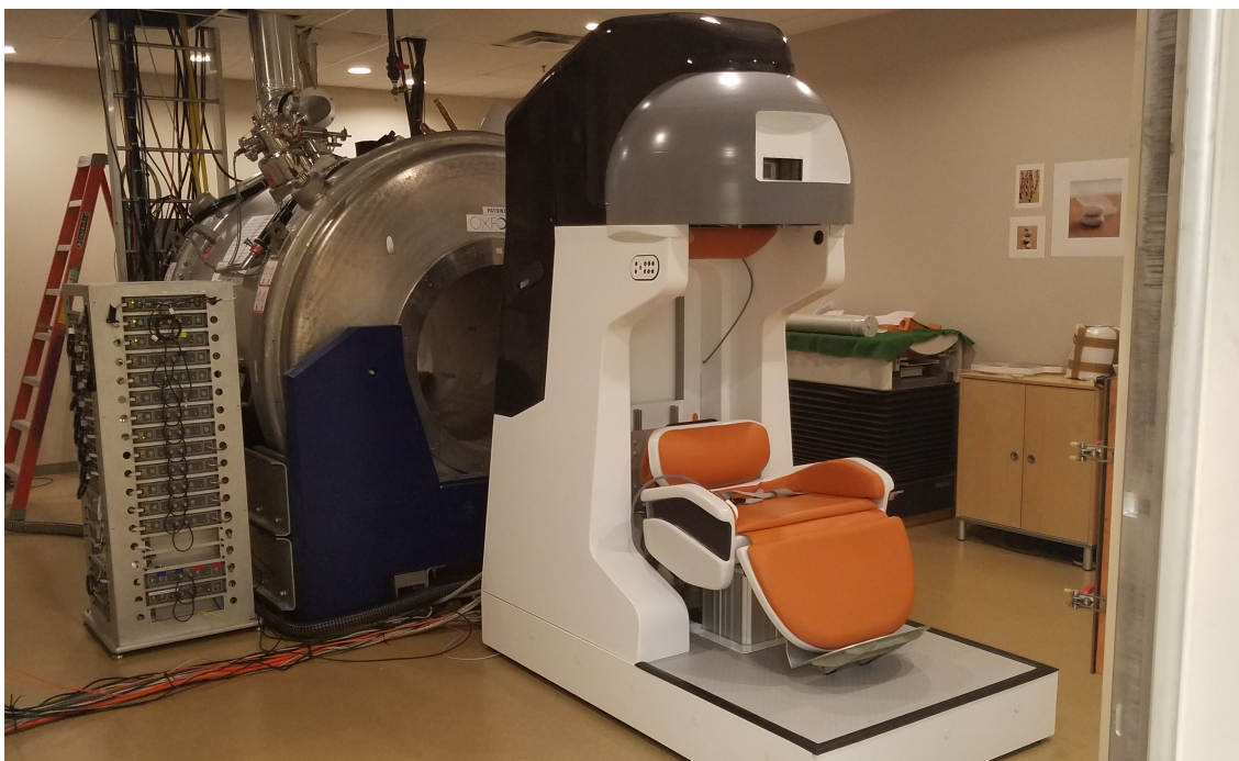
Fig. 5.3. Portable HTS magnet system installed at the Center for Magnetic Resonance Research. It was placed in front of a ramped down 4 T whole body scanner that utilized a low temperature superconductor and liquid helium to generate the main polarizing field. The silver hemisphere contains the HTS coils and generates the main polarizing field that a patient is raised into. The photo illustrates the stark contrast of the total size of the new portable scanner compared to the previous conventional system.
