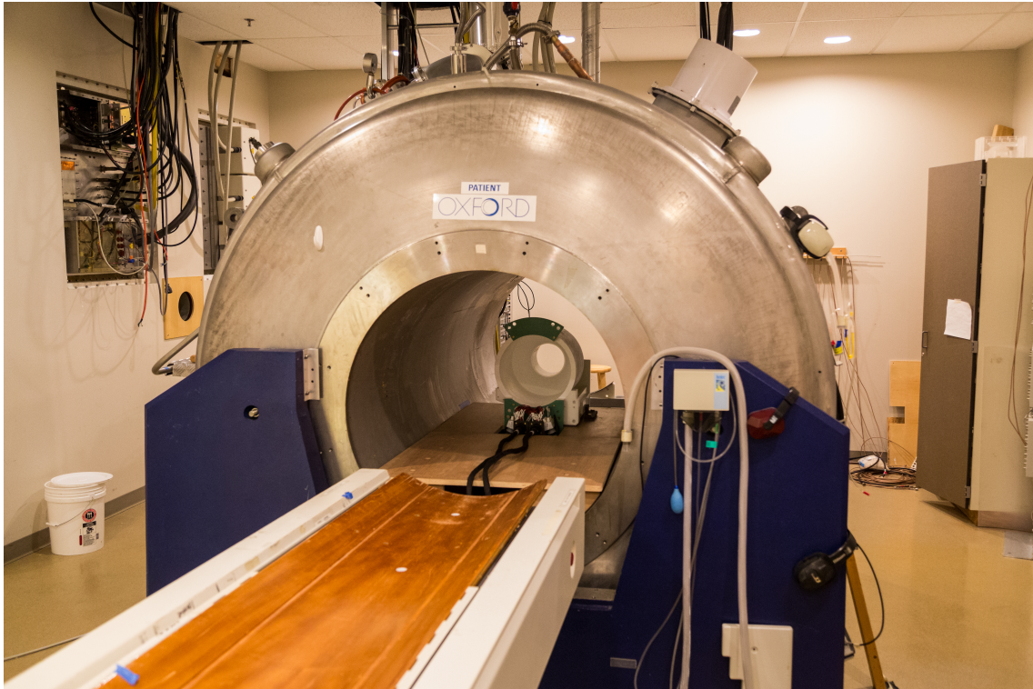
Fig. 5.1. MC-Array Mounted inside an Oxford 1.5 T whole body Magnet. A custom holder was designed and built to secure the MC-array at the isocenter of the magnet. All of the necessary plumbing and electrical connections were installed in place to better replicate the final installation within the portable magnet.
