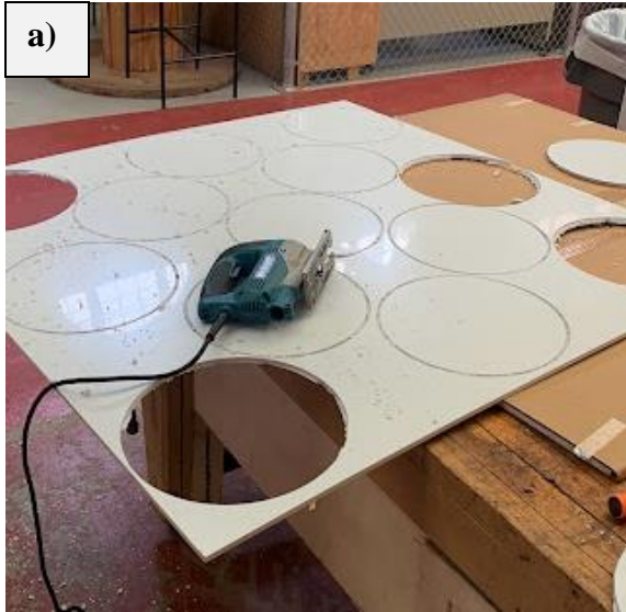
Figure 2.2: a) Cutting soil column baseplates from PVC board using a jigsaw. b) Shaping the soil column baseplate with a hand router.
