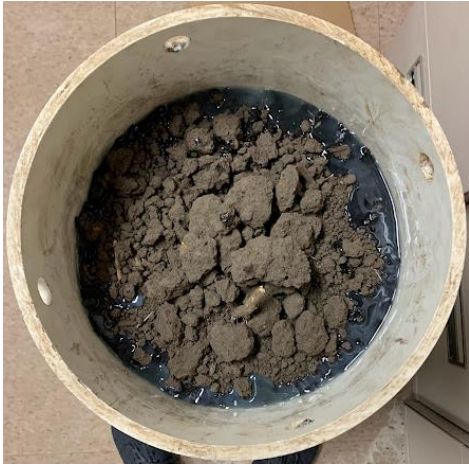
Figure 2.6: Liquified petroleum jelly surface applied around the circumference of the soil column to prevent sidewall flow of water during irrigation events.
