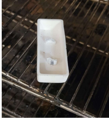
Figure 4.5: Trigger Material Oven Set-up Without Crucible Lid
