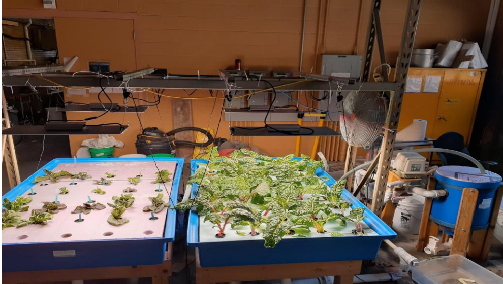
Figure 10: An image of both hydroponic production systems. The recirculation pump and reservoir are located on the far right. The growing area is approximately 1 x 1.5 m for each system.
