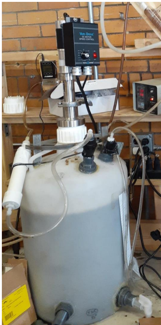
Figure 6: The 40 L AD vessel has an agitator, feeding port, sample port, heater, thermocouple, and gas port as shown above. The digester vessel is approximately 35 cm by 53 cm and the temperature is maintained at 35 C. Height is approximately a meter with the agitator.
