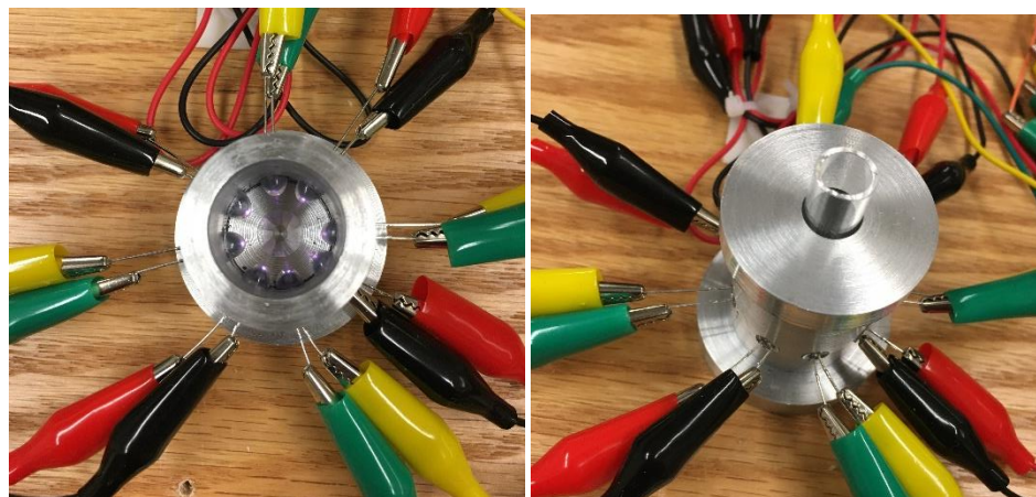
Figure S 7.8 Photolysis apparatus equipped with 8 350 nm LEDs arranged in a radial manner. Left: Apparatus without top. Right: Apparatus with top showing reaction tube inserted into the center.
