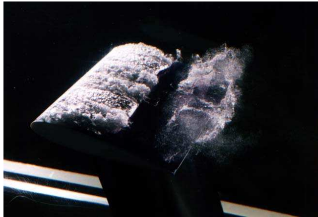
Figure 1.2: Sheet to cloud cavitation over a hydrofoil with a detached cloud cavity [8].
