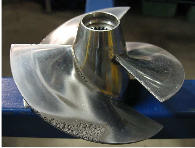
Figure 1.4: Example of material erosion due to cavitation [8].
