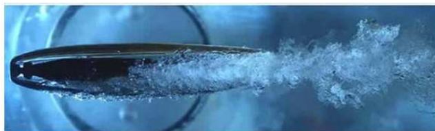
Figure 1.3: Example of supercavitation [9].
