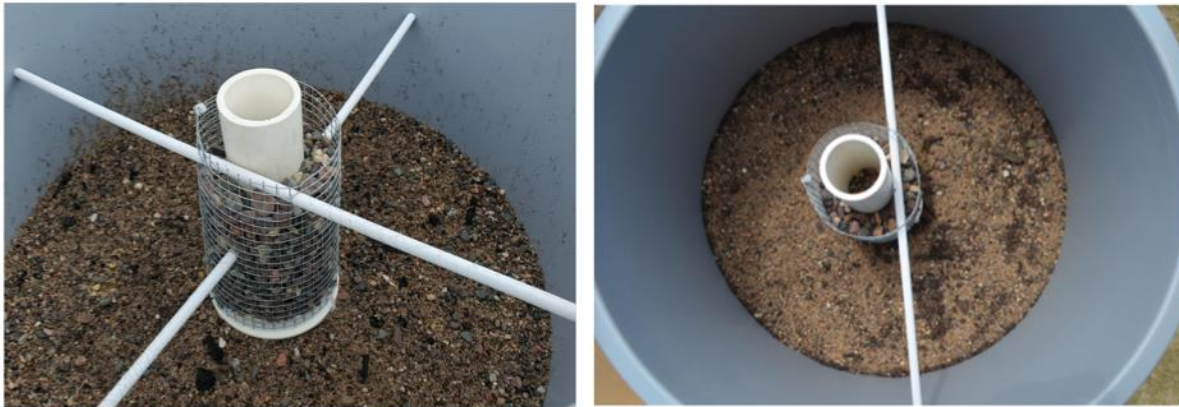
Figure 12: Side (left) and aerial (right) photos of dissipater columns.
