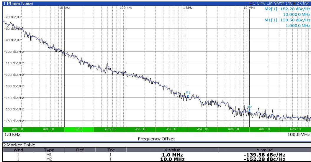
Figure 4.32: Measured phase noise spectrum of the input reference signal.
