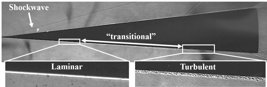
Figure 1.3: Laminar-turbulent transition on ballistic slender cone at Mach 4 [8].
