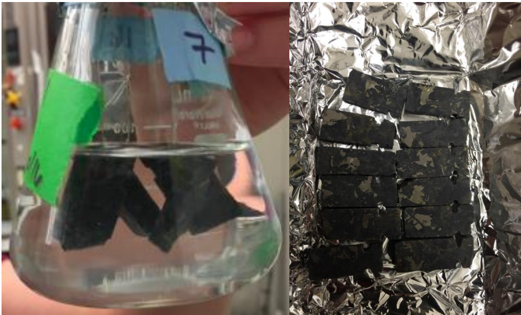
Figure C-2. Chips of ore-bearing Duluth Complex rock suspended in leaching media, and a close-up image of rock chip surfaces showing a mixture of sulfide minerals and silicate matrix.
