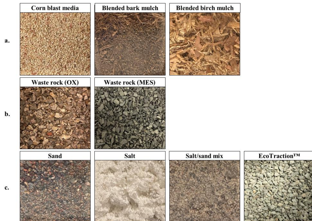
Figure 2. Project material used for evaluation. Local alternative abrasive materials were (a) mulches and corn grits as organic material and (b) mining waste rocks as inorganic materials. (c) Conventional materials and a traction salt-free alternative consumer product material were used for comparison.
