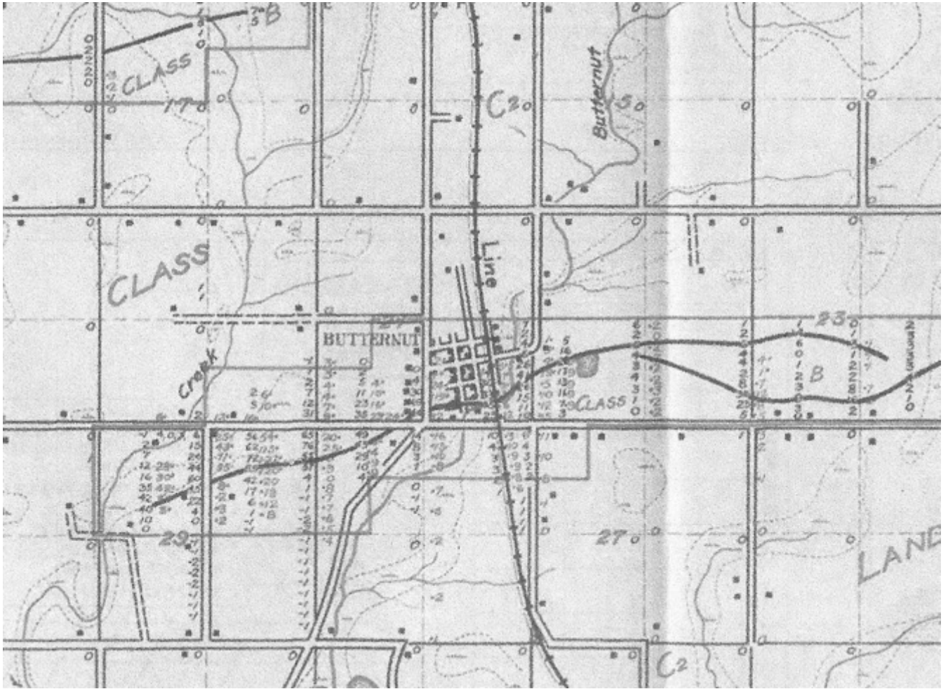
Figure 22. Magnetic observations in the Butternut (Ashland County), Wisconsin region (T.41N., R.1W.) associated with iron formation of the Turtle River Range that extends from this area ENE
