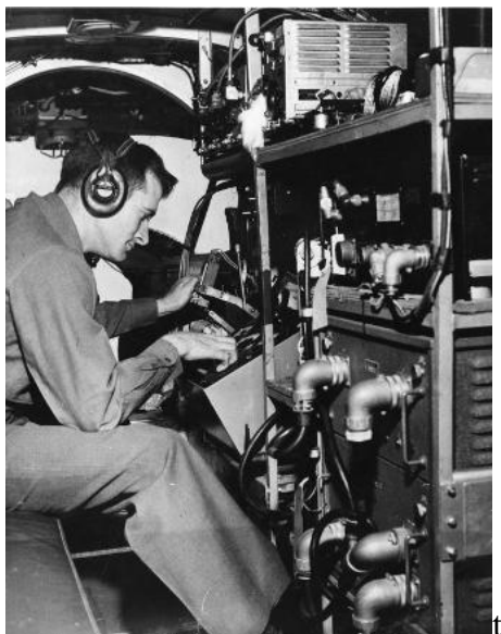
Figure 41. James R. Balsley (1916–1994) making magnetic observations in a U.S. Geological Survey aircraft. Balsley was among the first to recognize the importance of the airborne magnetometer in mapping geology, conducted some of the first aeromagnetic surveys, and
