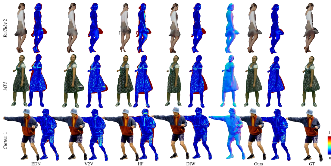
Figure 9.11. We compare our method to several baselines (EDN [26], V2V [27], HFMT [28], DIW [4]) on various sequences. For each example, we show the ground truth (GT) target appearance, the synthesized appearance by each method, and a color map of the error between the two. For our method, we also visualize the predicted surface normal.
