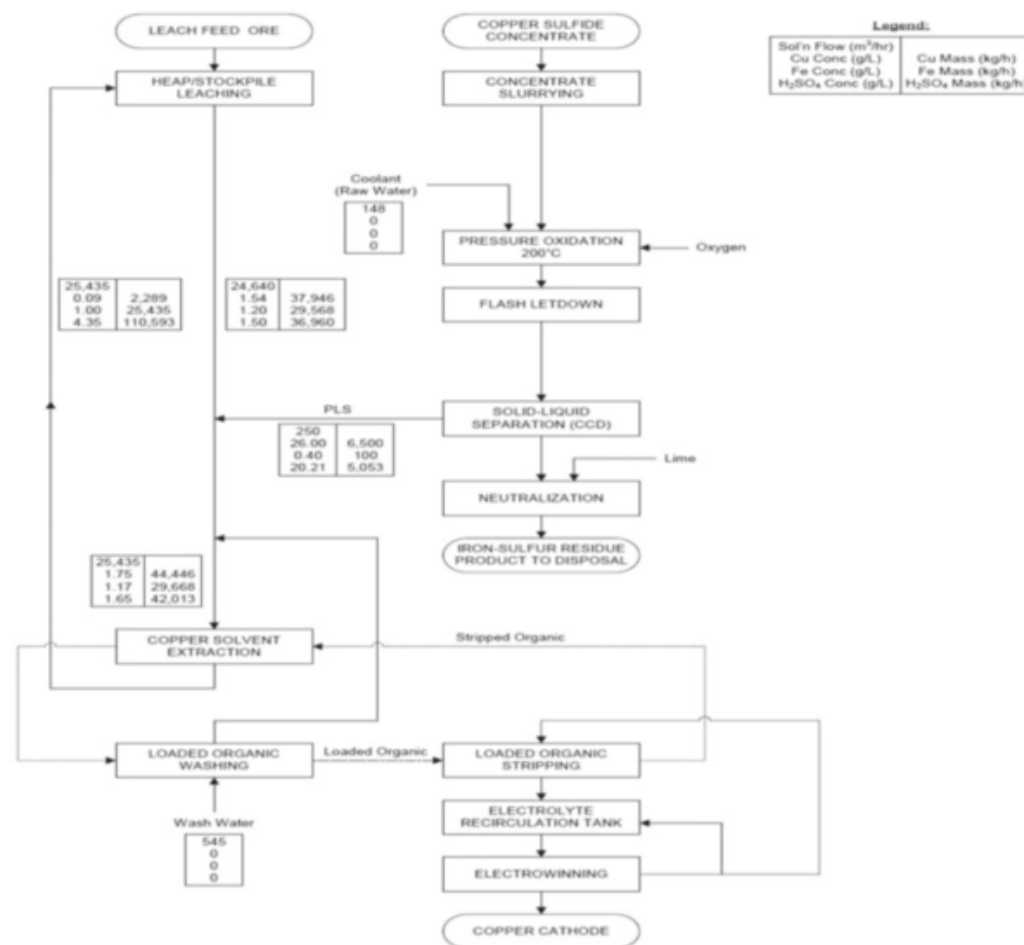
Figure 20. Medium-temperature pressure oxidation process practiced at Freeport McMoran's Morenci facility, AZ, USA (Source: Green, et al., 2018).
