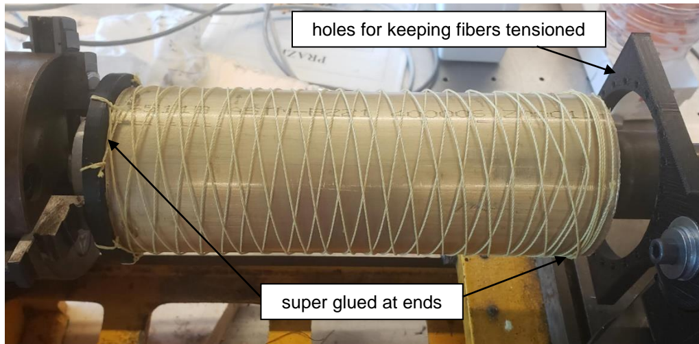
Figure 67: Completed fiber wrapping (all eight fibers)
