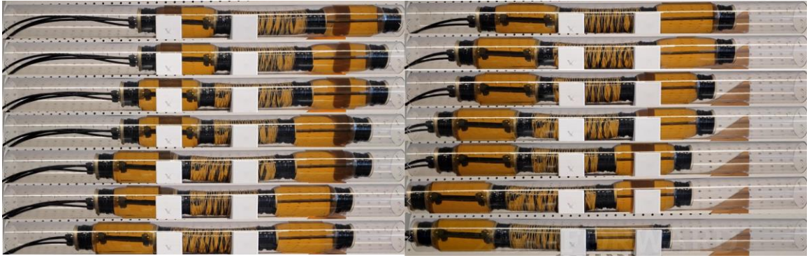
Figure 186: Multi-segment robot sequence through the 63.5 mm tube in the reverse direction
