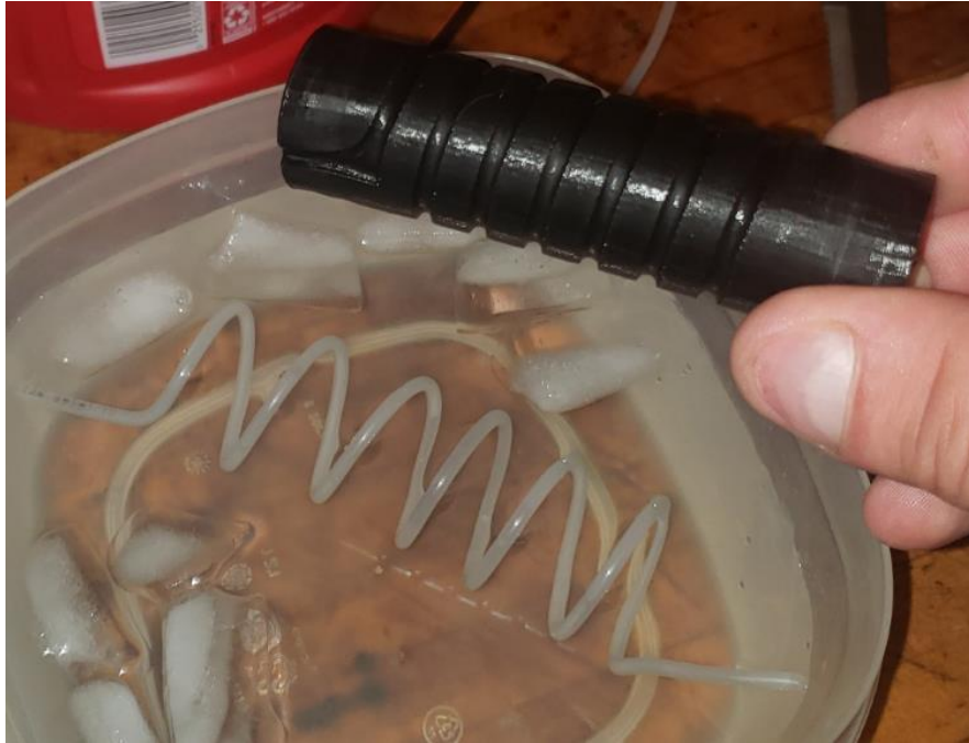
Figure 172: Microbore spiral removed from 3D printed mold after ice bath (note: different clear microbore tubing shown here)
