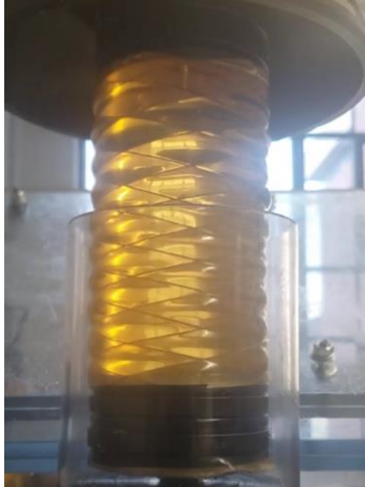
Figure 93: Bulging observed in Actuator 5 of the extending McKibben experiments
