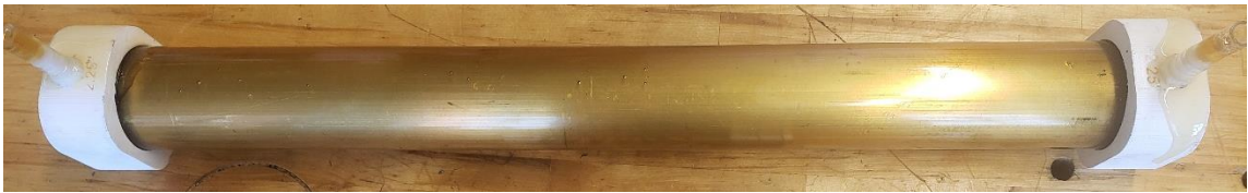
Figure 167: Injected elastomer in port block assembly
