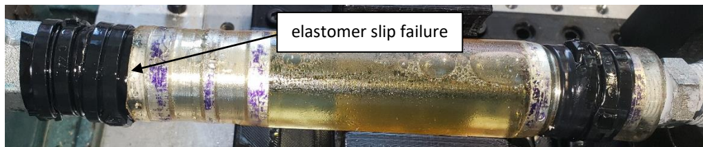
Figure 137: Traction Actuator 1A failure in 44.5 mm ID tube (insufficient clamping force led to elastomer slipping)
