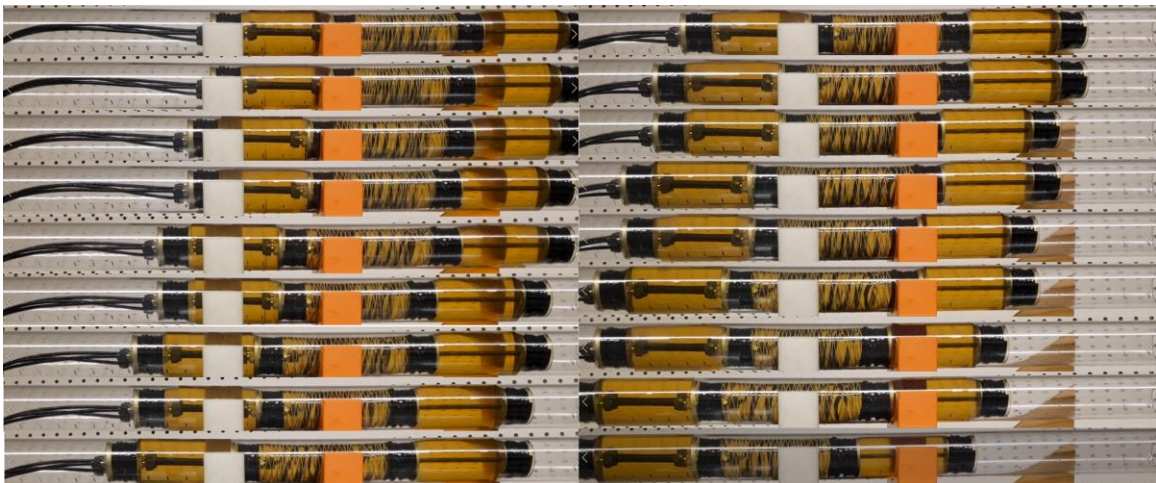
Figure 182: Multi-segment robot sequence through the 57.2 mm tube in the reverse direction
