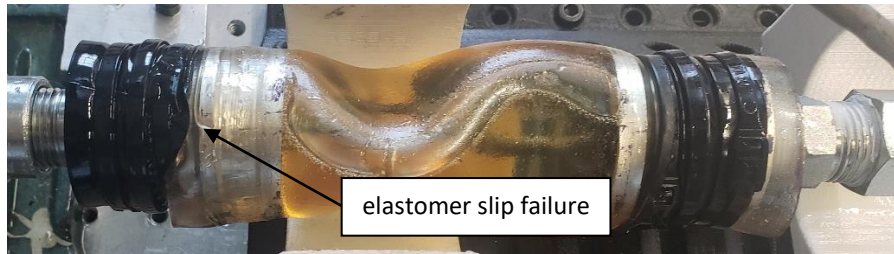
Figure 139: Traction Actuator 1C failure in 63.5 mm ID tube (insufficient clamping force led to elastomer slipping)
