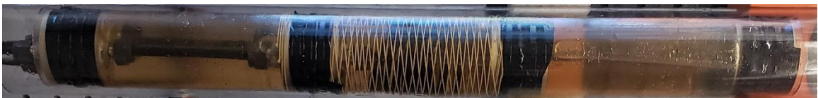
Figure 49: Finalized multi-segment soft robot
