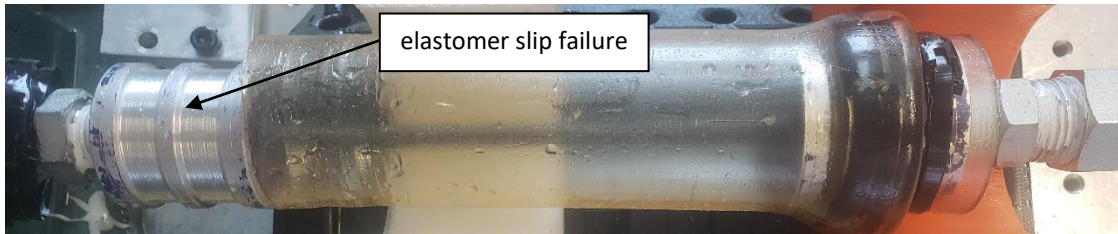
Figure 143: Traction Actuator 2C failure in 57.2 mm ID tube (insufficient clamping force led to elastomer slipping)
