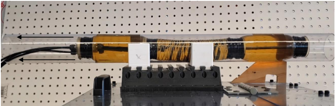
Figure 185: Multi-segment robot halfway through the 63.5 mm tube in the reverse direction
