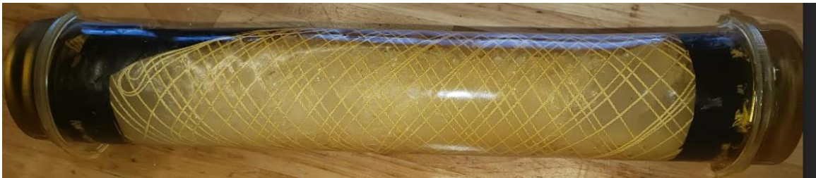
Figure 119: Dual elastomer layer CaCl expanded traction segment
