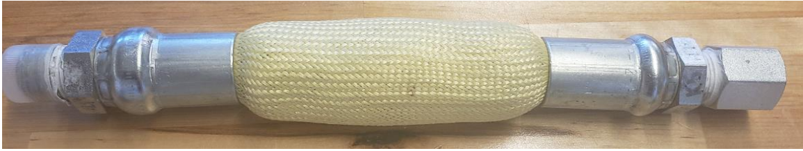
Figure 118: Modified McKibben actuator with loose fiber sleeve and internal threaded rod
