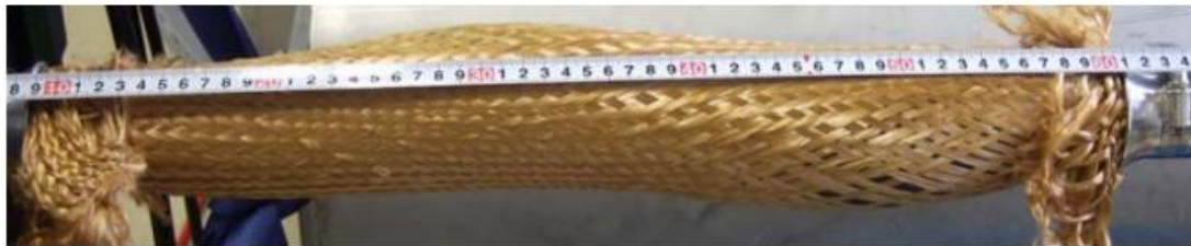
Figure 17: Fiber sleeve loosening [64]
