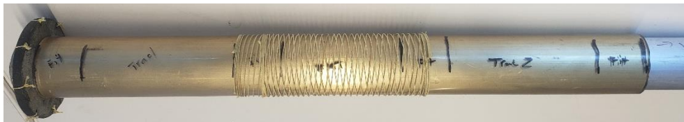
Figure 170: Completed fiber-wrapped elastomer
