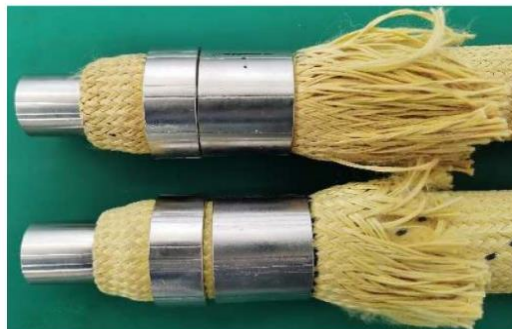
Figure 18: Segment connector slipping [64]
