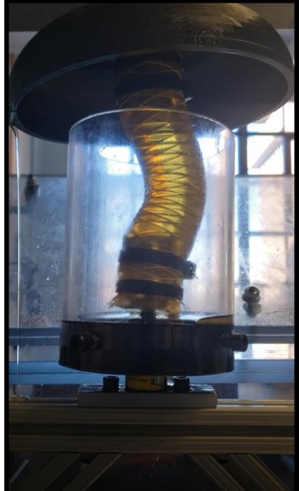
Figure 105: Pressurized accelerated buckling failure
