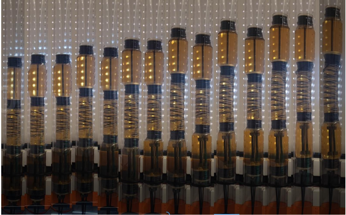
Figure 188: Multi-segment robot sequence through the 63.5 mm tube in the vertical orientation
