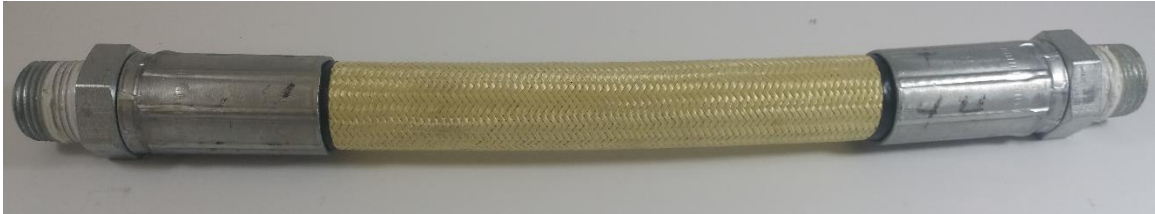
Figure 53: Fabricated McKibben actuator with crimped fitting (Actuator D)
