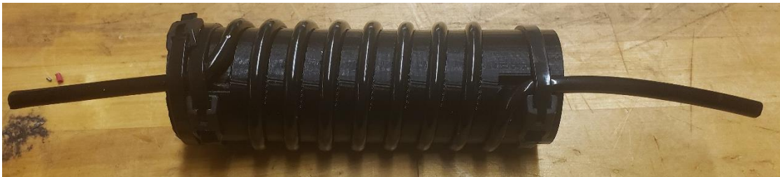
Figure 171: Microbore tube spiral zip tied to 3D printed mold
