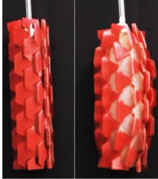
Figure 116: Kirigami skin applied to radially expanding, axially contracting McKibben actuator to improve traction force generation [127]
