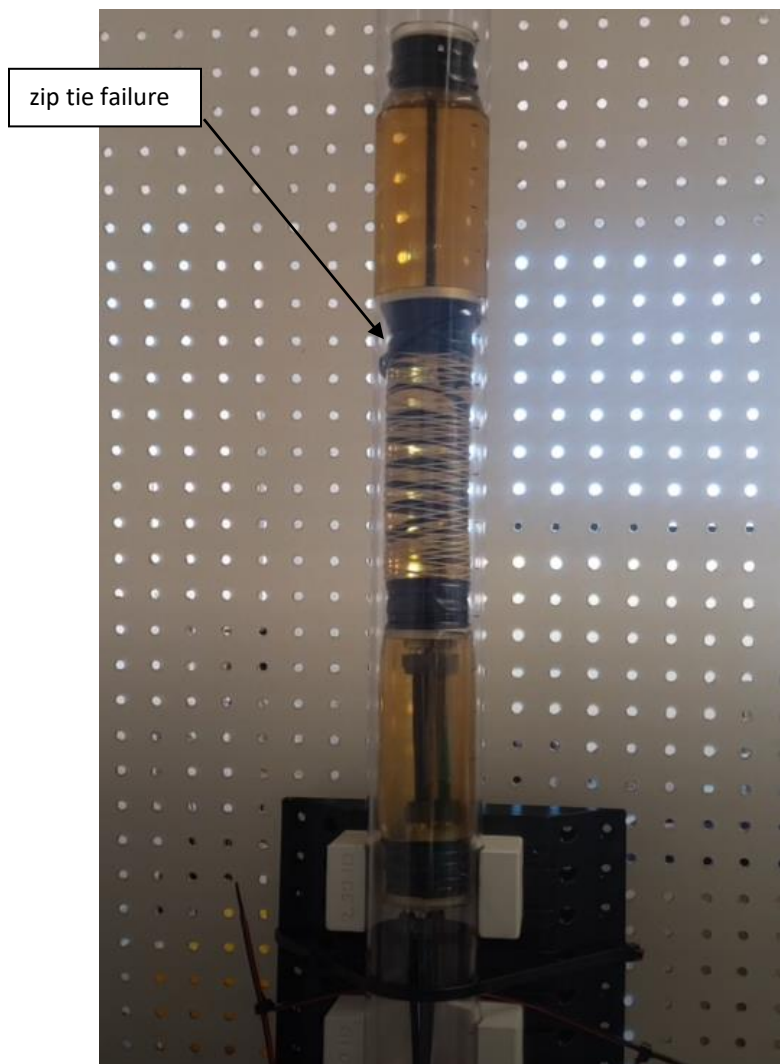
Figure 189: Zip tie failure at segment connector between extender and distal traction segment
