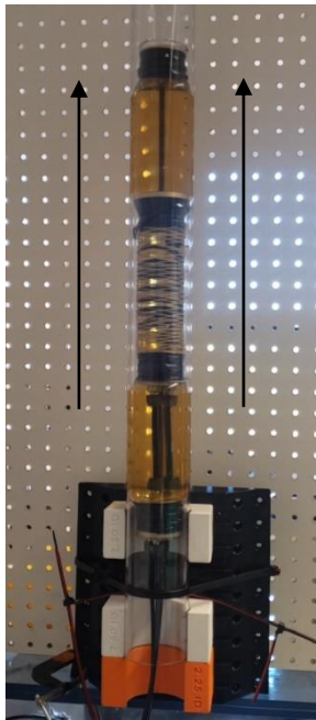
Figure 187: Multi-segment robot halfway up through the vertical 63.5 mm tube in the forward direction
