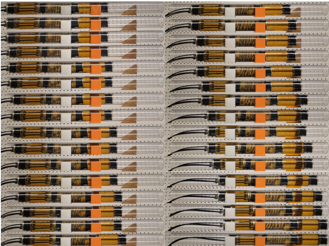
Figure 180: Multi-segment robot sequence through the 57.2 mm tube in the forward direction
