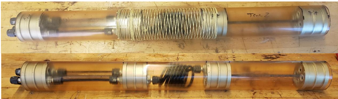
Figure 174: Completed multi-segment robot before electrical tape and zip ties are applied (top: with fibers, bottom: without fibers)
