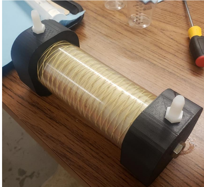
Figure 68: Completed elastomer with fibers sandwiched between layers
