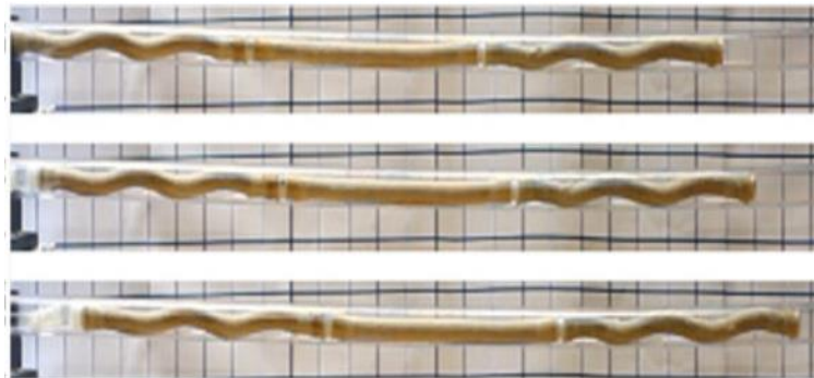
Figure 38: Pneumatic, serially-actuated multi-segment tube traversing robot [109]
