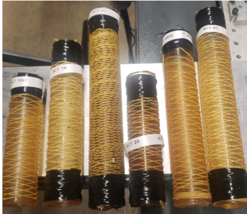
Figure 99: Wrapped elastomers for buckling experiments
