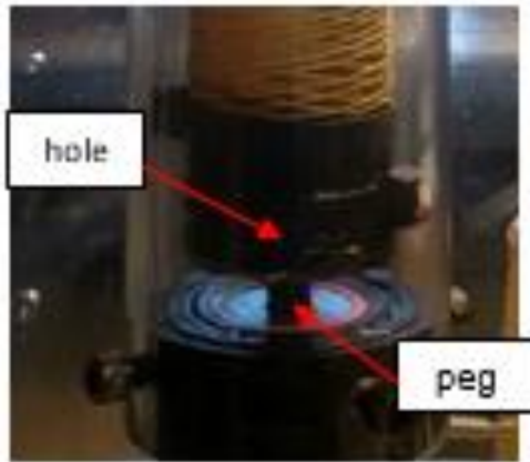
Figure 100: Actuator engaged with load-cell peg
