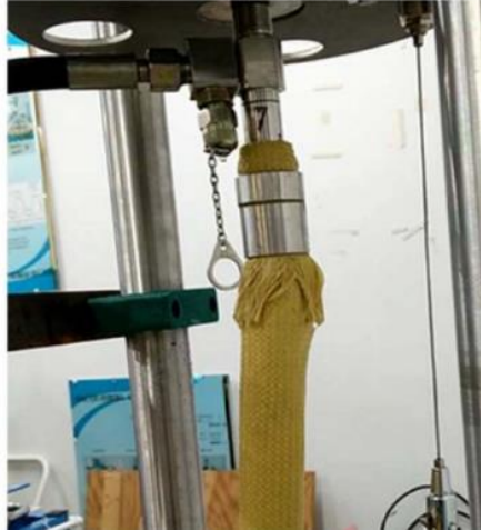
Figure 19: Elastomer slipping out of connector [64]
