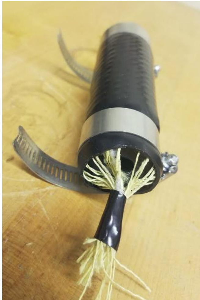
Figure 215: Fiber wrapped elastomer coated with polyvinylchloride heat shrink tubing
