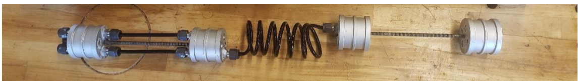
Figure 173: Completed internal structure of multi-segment robot
