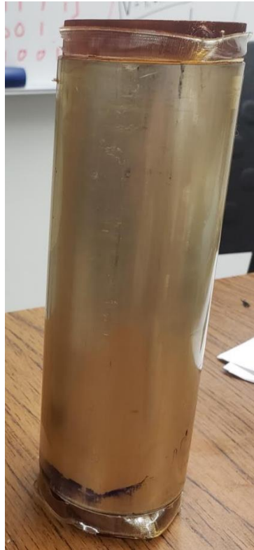
Figure 65: Elastomer on outside surface of aluminum rod
