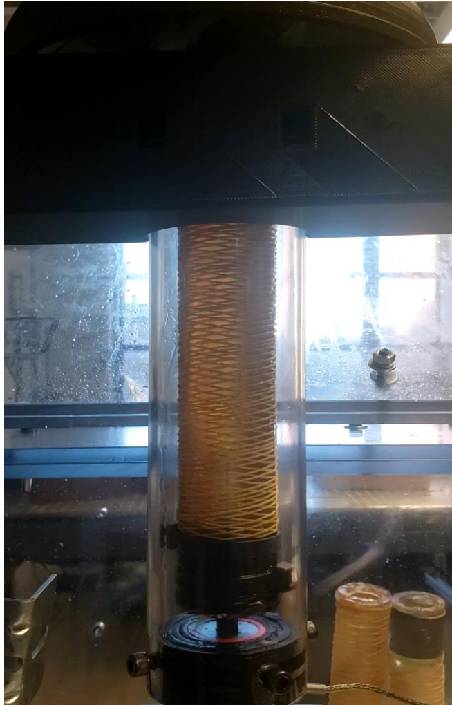
Figure 103: Extending McKibben actuator in experimental apparatus
