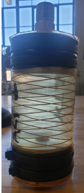
Figure 22: Custom fiber-wrapped McKibben actuator developed by the author
