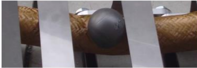
Figure 51: Hydraulic McKibben burst failure [21]
