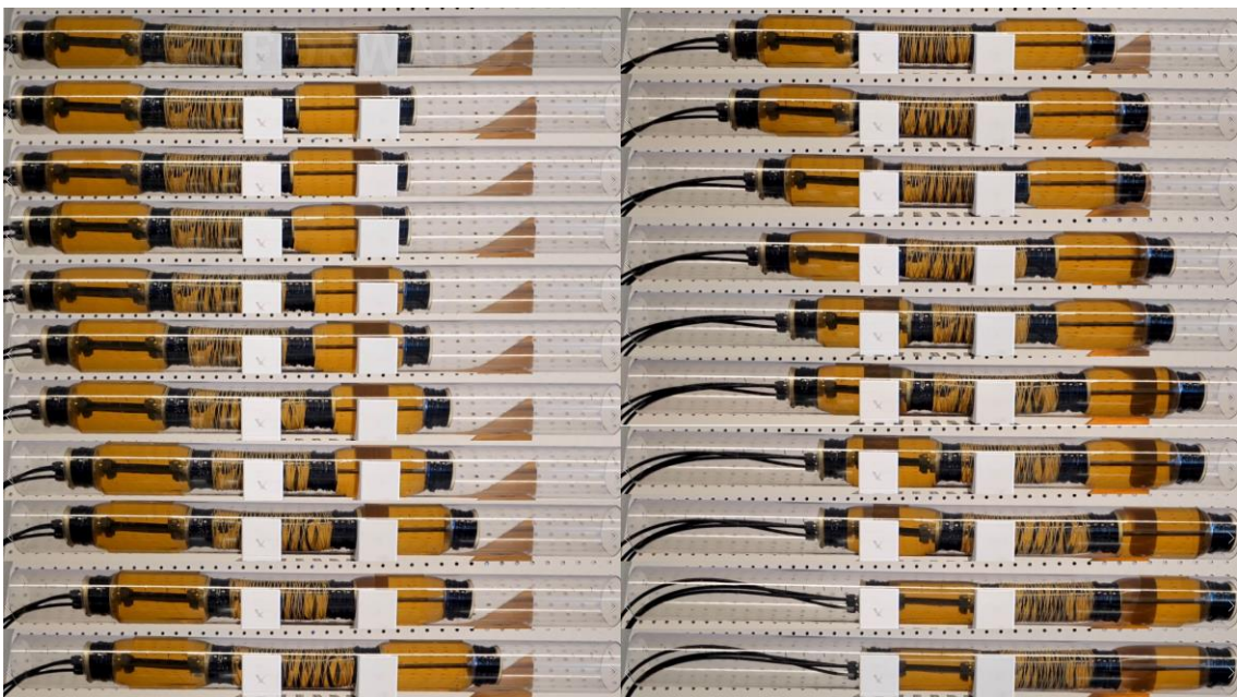
Figure 184: Multi-segment robot sequence through the 63.5 mm tube in the forward direction
