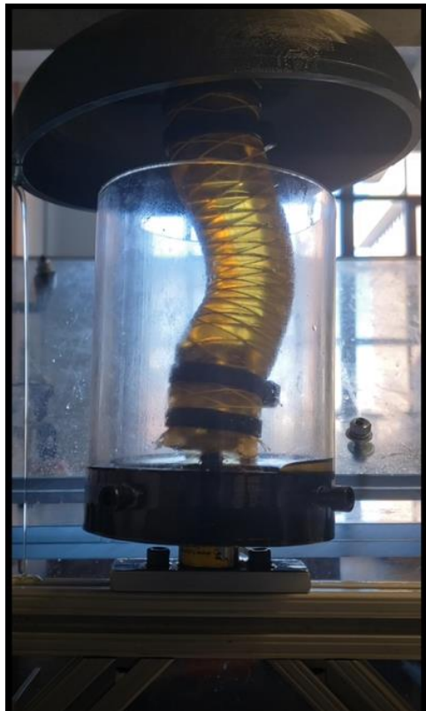
Figure 25: Buckling McKibben actuator developed by the author
