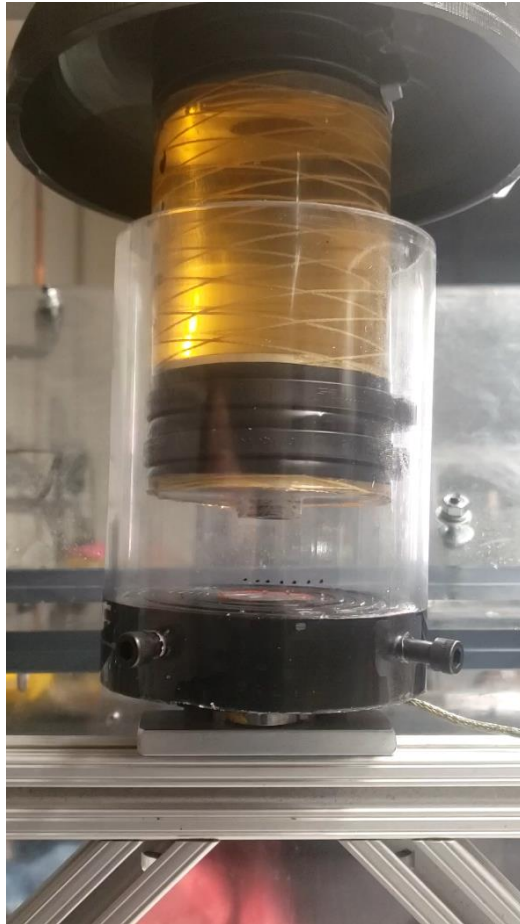
Figure 73: Side view of extending actuator, adjustable cross bar, and load cell
