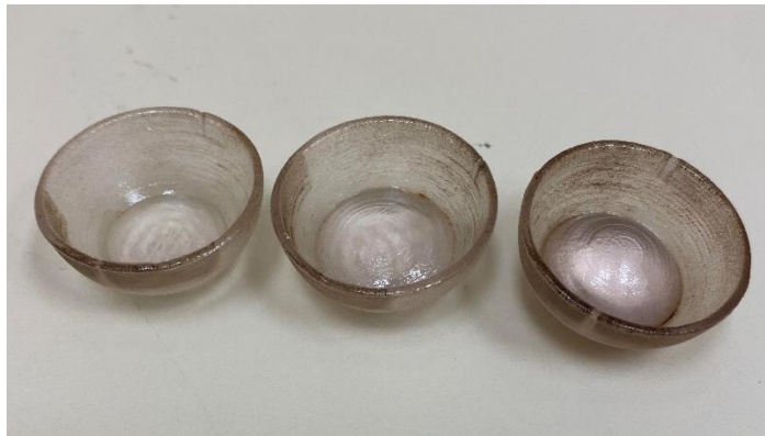
Figure 2.6 3D-Printed Eye Phantoms with Increasing Tumor Heights
