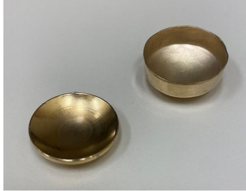
Figure 2.1 Custom NdFeB Magnet and 20 mm COMS Plaque with Adjusted Lip Height
