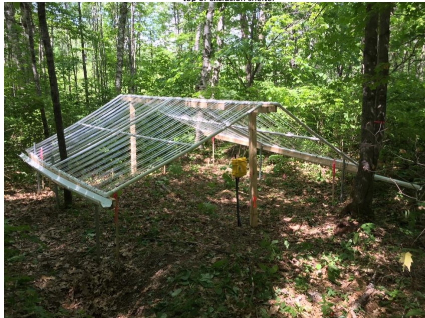
Figure 2.3: Paired-plot design with throughfall reduction treatment during the growing season. All plots and transparent roof panels are oriented on an east-west transect, with the ridgeline of shelter running north-south. Precipitation reduction shelters are designed to exclude 50% of throughfall. Plots that received treatment were randomized in each pair. The bottom photo shows the throughfall exclusion shelter on a treatment plot during the growing season. (Photo credit: Alan Toczydlowski)
