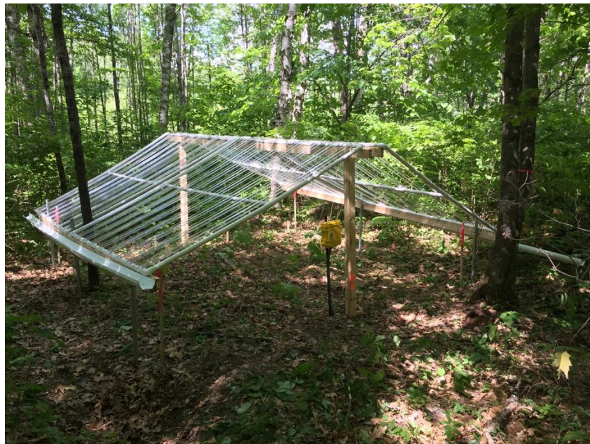
Figure 1.3: Paired-plot design with precipitation reduction treatment during the growing season. All plots and transparent roof panels were oriented on an east-west transect, with the ridgeline of the shelter running north-south. Precipitation reduction shelters were designed to exclude 50% of throughfall. Plots that received treatment were randomized in each pair. The bottom photo shows the throughfall reduction shelter on a treatment plot during the growing season. (Photo credit: Alan Toczydlowski)
