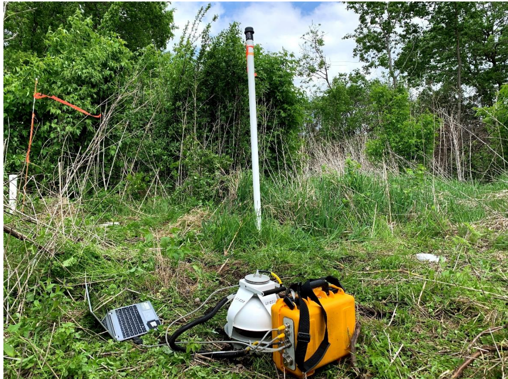
Figure 14: Measuring flux with LICOR LI-1800A near well CSA at Cold Spring fen
