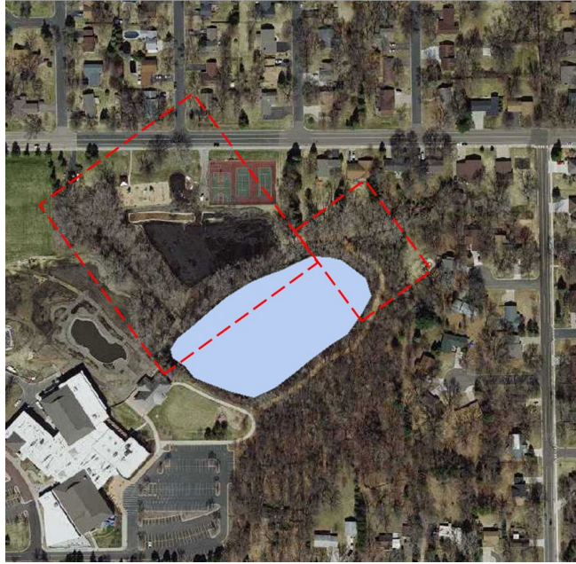
Figure 26. Conceptual diagram of the Case C potential tree removal scenario for the Shoreview pond. This scenario expands the tree removal area to encompass the northern half of the pond with limited tree removal adjacent to residential properties.
