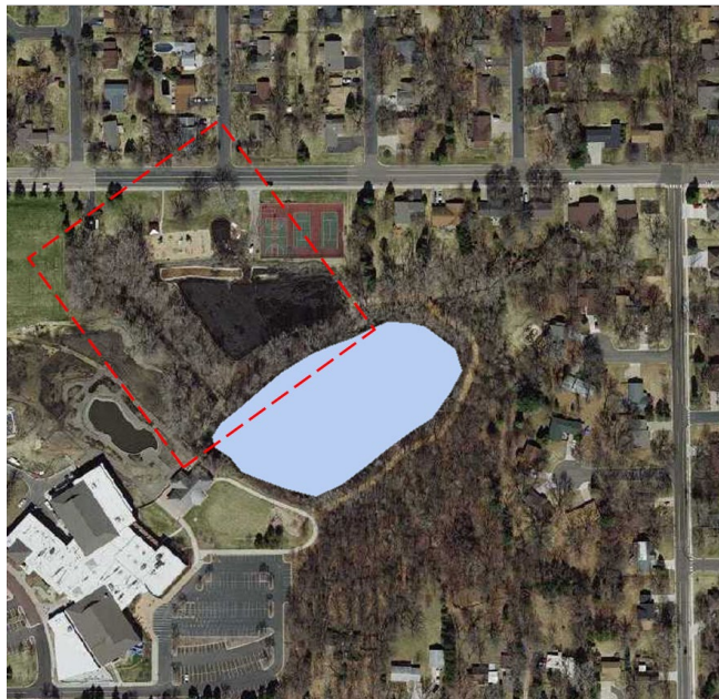
Figure 25. Conceptual diagram of the Case B potential tree removal scenario for the Shoreview pond. This scenario more broadly exposes the pond to winds from the northern and western directions by removing a large swath of trees that are not adjacent to residential properties.
