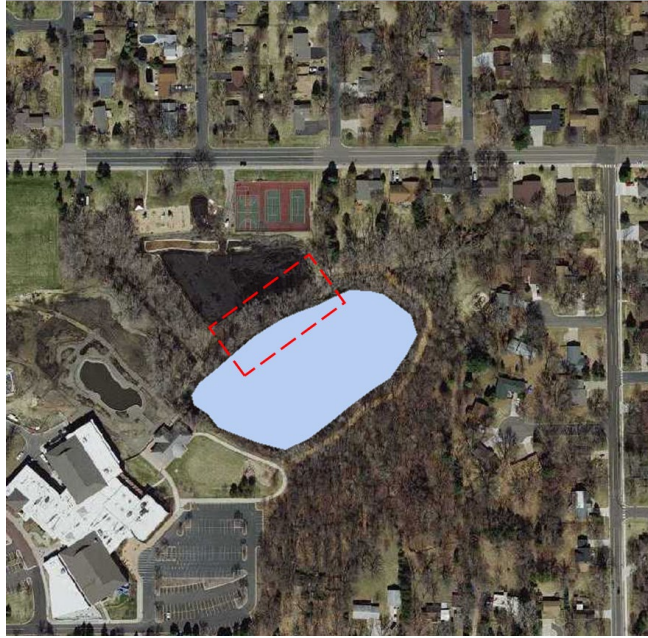
Figure 24. Conceptual diagram of the Case A potential tree removal scenario for the Shoreview pond. This scenario targets a thin line of trees shielding the pond from the direction of prevailing wind (northwest).
