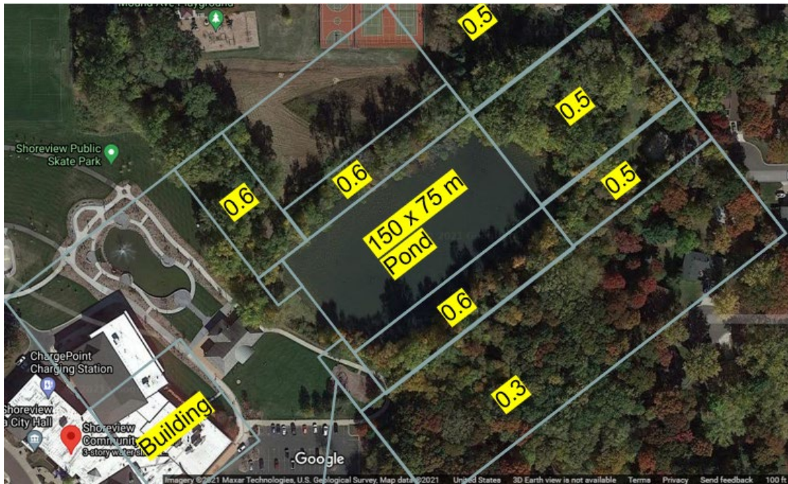
Figure 22. Conceptual diagram of wind sheltering grid in ANSYS-Fluent. The highlighted numbers (0.3, 0.5, 0.6) represent the relative tree densities input to the Fluent model.
