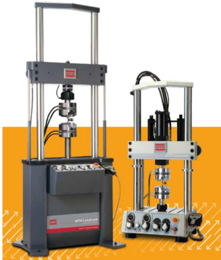
Figure 1.2 Loadframes: These are two varieties of loadframes. The loadframe on the left is a 370.10 model with a frame and actuator rated for 100kN with a servovalve which has flow rating of 15gpm at 1000psi. The loadframe on the right is a 370.02 model, which has a frame and actuator rates for 25kN of force and a servovalve which has a flow rating of 5gpm at 1000psi. [3]
