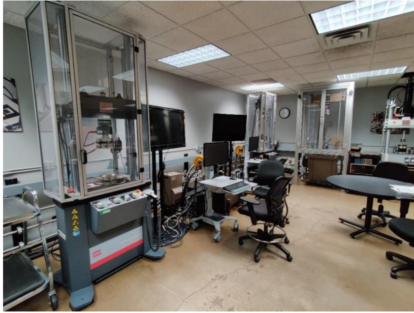
Figure 2.4 MTS Lab setup: A materials testing lab with three loadframes connected a hardline that run along the wall connecting them to the pump in the far corner of the room (Figure 2.5)
