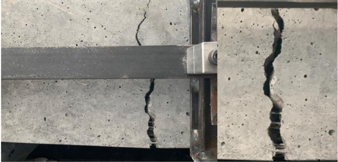
Figure 4-15. Fibers bridging a crack during an ongoing four-point flexural bending test.
