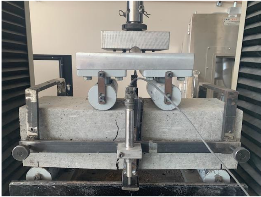
Figure 4-14. Four-point flexural bending test as per ASTM C 1609
