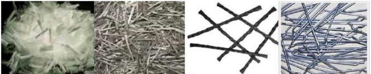
Figure 2-18: Fibers used in the (Kevern et al., 2016) study: polypropylene fibrillated fiber (left), polypropylene macro fiber (left middle), carbon fiber (right middle) and steel fiber (right)
