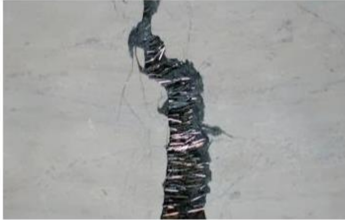
Figure 2-11. Crack control and bridging effect of fibers (Gaddam, 2016)
