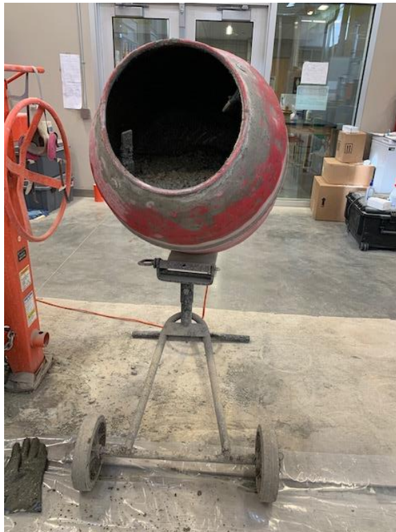
Figure 4-6. Concrete mixer used.
