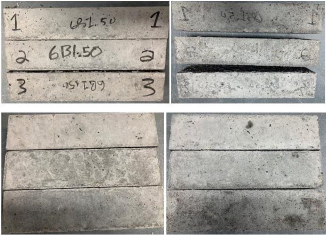
Figure 0-32. Before (Left) and After (Right) image of mix 6B1.50 beams subjected to 300 freeze-thaw cycles
