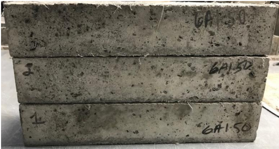
Figure 0-33. Image of mix 6A1.50 beams after 300 freeze-thaw cycles
