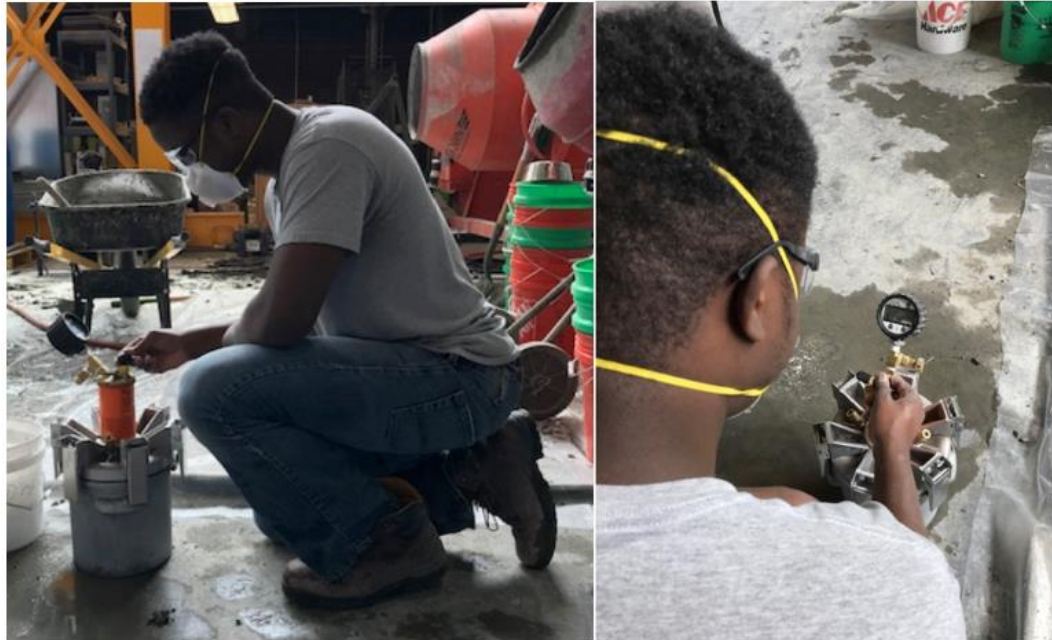
Figure 4-8. Ongoing SAM test
