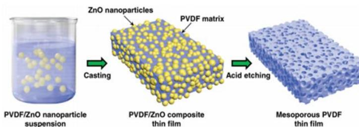
Figure 5. PVDF fabrication with ZnO nanoparticles<sup>11</sup>. The ZnO nanoparticles are added to a solution of PVDF dissolved in 2-butanone. This suspension is then cast into a petri dish and the 2-butanone is evaporated off leaving a PVDF/ZnO composite thin film. After being placed in an acid bath, a spongelike mesoporous PVDF thin film is left.
