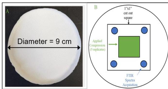
Figure 6. Fabricated PVDF sample. Image A shows a fabricated PVDF sensor. Image B shows where the compression force was applied and where the FTIR spectra was collected on the 1"x1" square.
