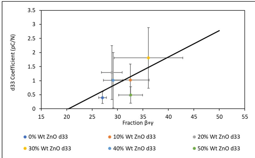
Figure 19.  $d_{33}$  values of 2 stacks of fabricated PVDF sensors compared to fraction of  $\beta$  and  $\gamma$  chain conformations. The black line indicates a trendline of increasing  $d_{33}$  values with increasing of  $\beta$  and  $\gamma$  chain conformations. The error bars show the standard deviation of the  $d_{33}$  values, and the standard deviation of chain conformations.
