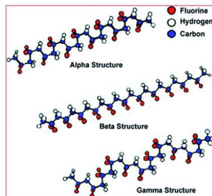
Figure 2. Different chain conformations of PVDF<sup>10</sup>.
