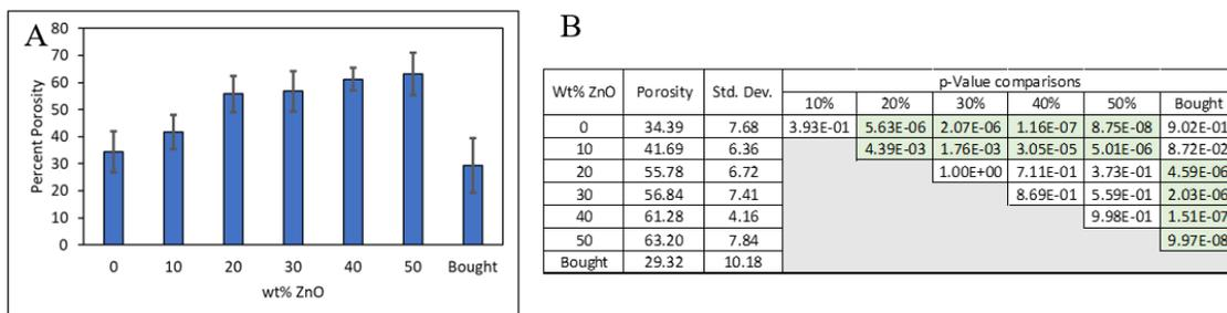
Figure 15. Percent Porosity of Fabricated and Bought PVDF sensors.  $n=8$  for fabricated PVDF sensors and  $n=4$  for bought PVDF samples. P-Value comparisons highlighted in green are significant at  $p<0.05$ .
