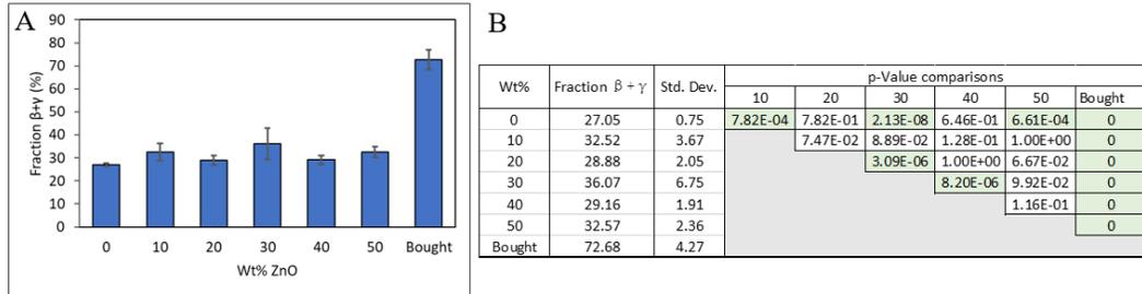
Figure 16. Chain conformations of PVDF Polymer. The fraction of  $\beta$  and  $\gamma$  chain conformations in the PVDF sensors is shown above in A. The “Bought” PVDF had the largest fraction at 72.6%, which is double the highest of the fabricated PVDF sensors which was 30%Wt ZnO.  $n=16$  for each type of sample. The p-value comparisons are shown in B. The green highlights significance at  $p < 0.05$ .
