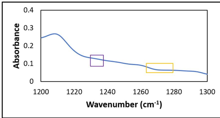
Figure 9. FTIR spectra for calculating the  $\beta$  and  $\gamma$  phases of PVDF. The yellow box shows the region of spectra for  $\beta$  phase chain conformation calculations outlined in equation 3. The purple box shows the region for  $\gamma$  phase calculations using equation 4.
