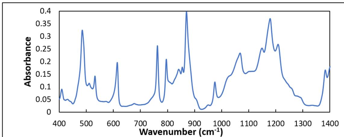
Figure 7. Whole FTIR Spectra of PVDF sensor.
