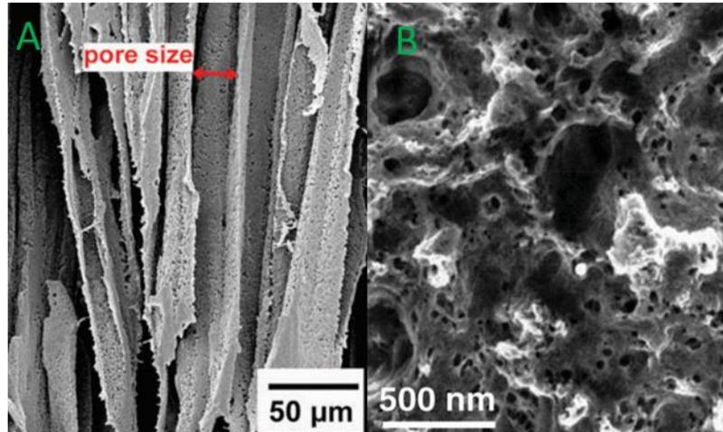
Figure 4. Porous PVDF Samples. Image A shows the scanning electron microscope image of an ice templated PVDF sample with lateral pores<sup>12</sup>. Image B shows a porous PVDF samples made from adding and removing ZnO nanoparticles during the fabrication process<sup>11</sup>
