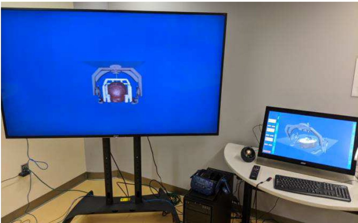
Figure 57. One VR design configuration for the DBS use case a 75" SWD (left) and a 24" touch screen (right). Users position the touch screen in front or next to the stereoscopic screen based on their preferences.
