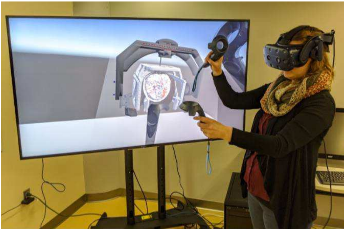
Figure 63. The second VR tool design for DBS procedural planning using an HMD.
