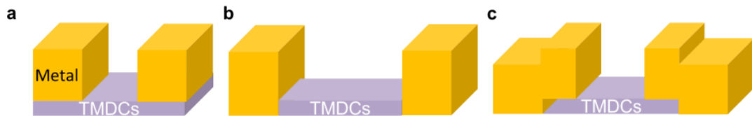
Figure 1.18: Contact topologies between bulk metals and 2D TMDCs. (a) top contact, (b) edge contact, and (c) combined contact.
