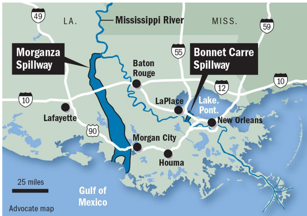
Figure 25. A map of the two primary spillways in South Louisiana; the Bonnet Carré and Morganza spillways. The original caption reads: “The Morganza Floodway is located at river mile 280 in central Louisiana. It is 186 river miles above New Orleans on the west bank of the river in Pointe Coupee Parish. It begins at the Mississippi River and extends southward to the East Atchafalaya River. It ultimately meets the Atchafalaya River Basin Floodway near Krotz Springs” (Advocate staff 2019).
