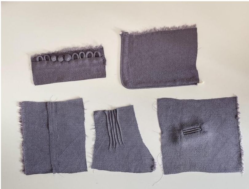
Figure 10: Selected Dress B fashion-fabric samples. Clockwise from top left - Loops and buttons, corded piping on a corner, jetted-pocket, shoulder pintucks, plain seam.
