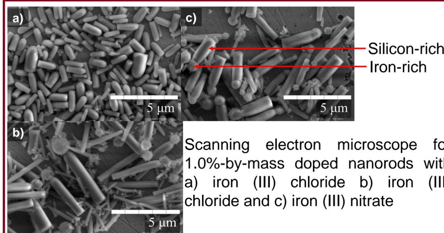
Scanning electron microscope for 1.0%-by-mass doped nanorods with a) iron (III) chloride b) iron (III) chloride and c) iron (III) nitrate
