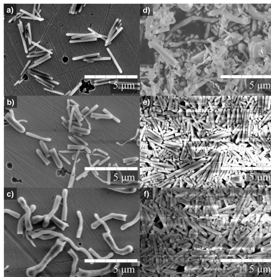
Scanning electron microscopy for nanorods synthesized from a) pure pentanol, and 1:4 ratio alcohol mixtures of b) ethanol to 1-pentanol, c) 1-propanol to 1-pentanol, d) 1-butanol to 1-pentanol e) 1-hexanol to 1-pentanol, f) 1-octanol to 1-pentanol
