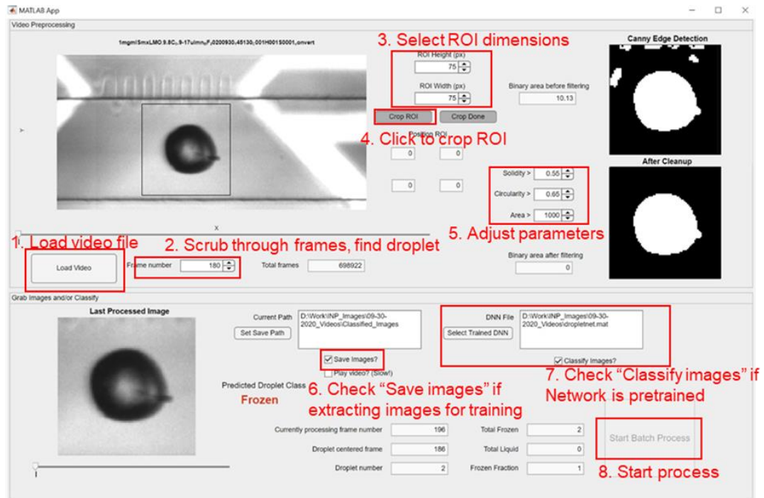
Figure E-1: MATLAB GUI app to crop video, extract droplet images and classify them using a DNN.
