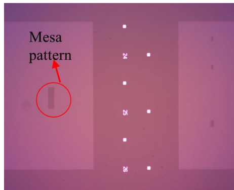
Figure 3.3. Optical micrograph showing patterns after mesa isolation etch and some alignment marks. The square alignment marks are of the size 20 \times 20 \mu\text{m}^2 .
