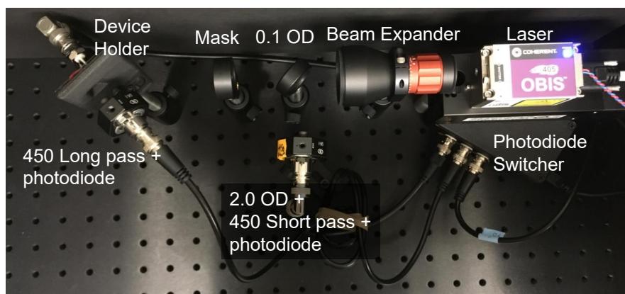
Fig. F.1. Experimental layout for EL photodegradation measurement.
