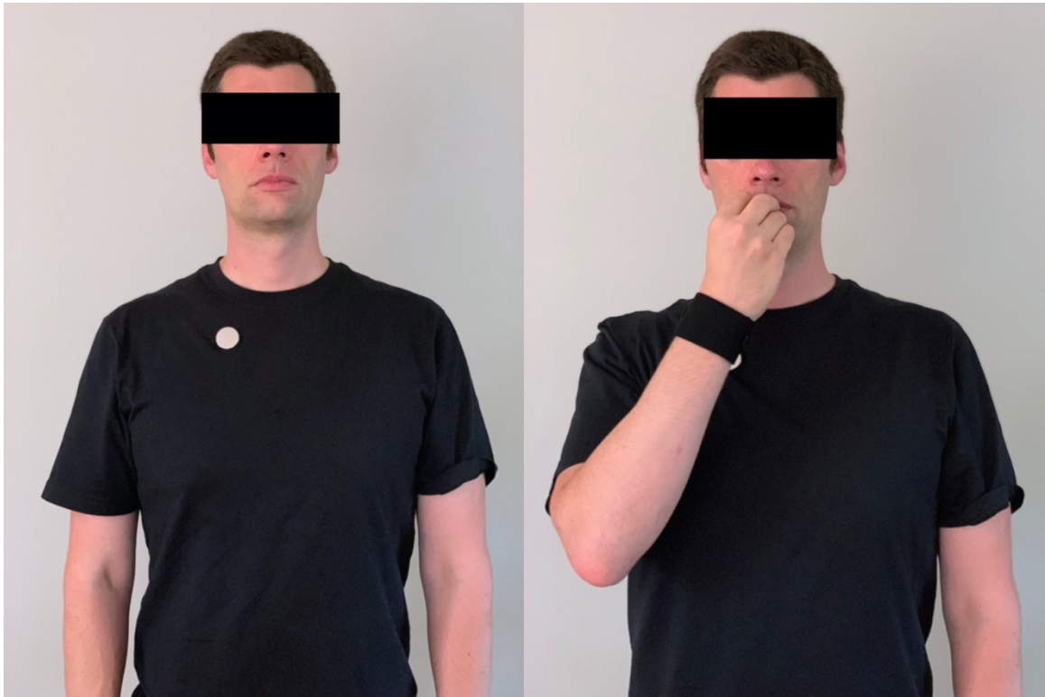
Fig. 32. Permanent magnet for hand-to-mouth proximity detection
